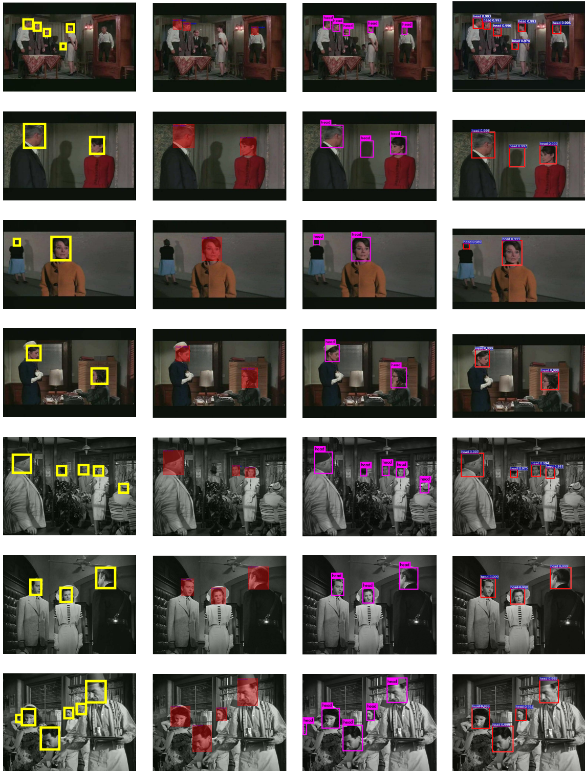
Figure 3.11: Qualitative Results: The first column shows the sample frames from test sequences overlaid with the ground-truth annotations. The second, third and fourth column shows the detection results using models fine-tuned on SSD MultiBox [101], YOLO [140] and Faster R-CNN [143] respectively. The rows from 1 – 4 and 5 – 7 show the results from Hollywood-Heads [181] and Casablanca [144] respectively. (Best viewed in colour)
