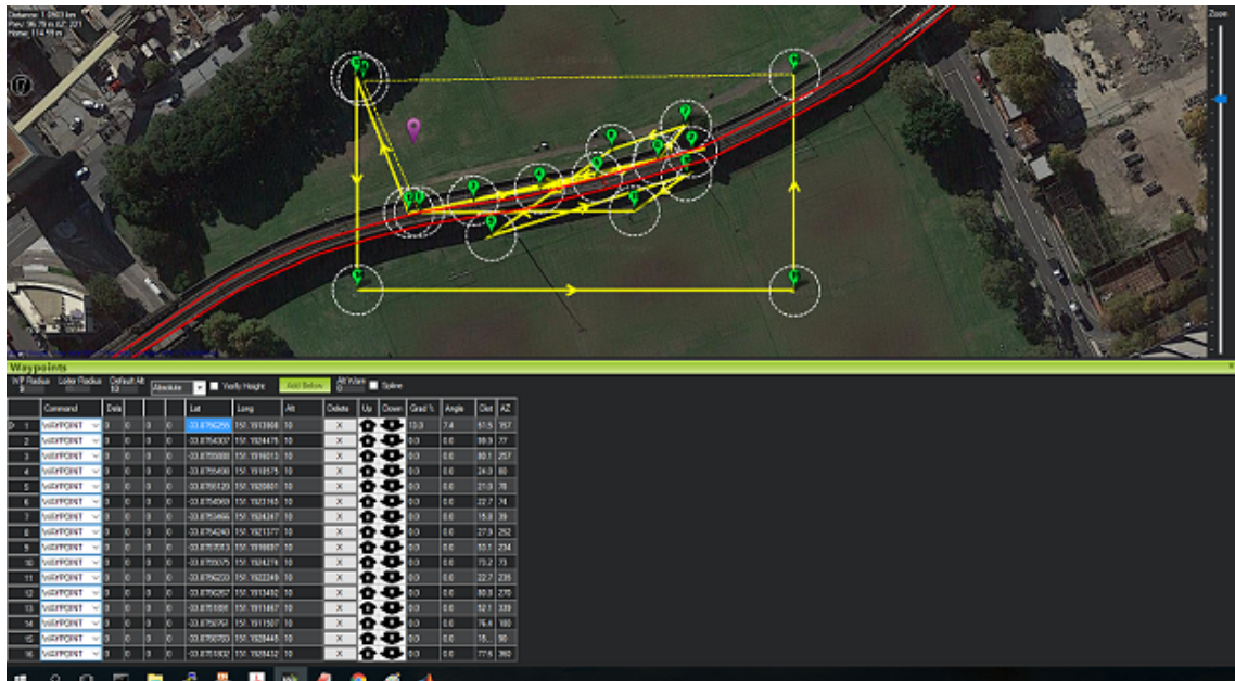
Figure 5.2 : Mission Planner incorporating Google Satellite Map to create initial information and an inspection plan
