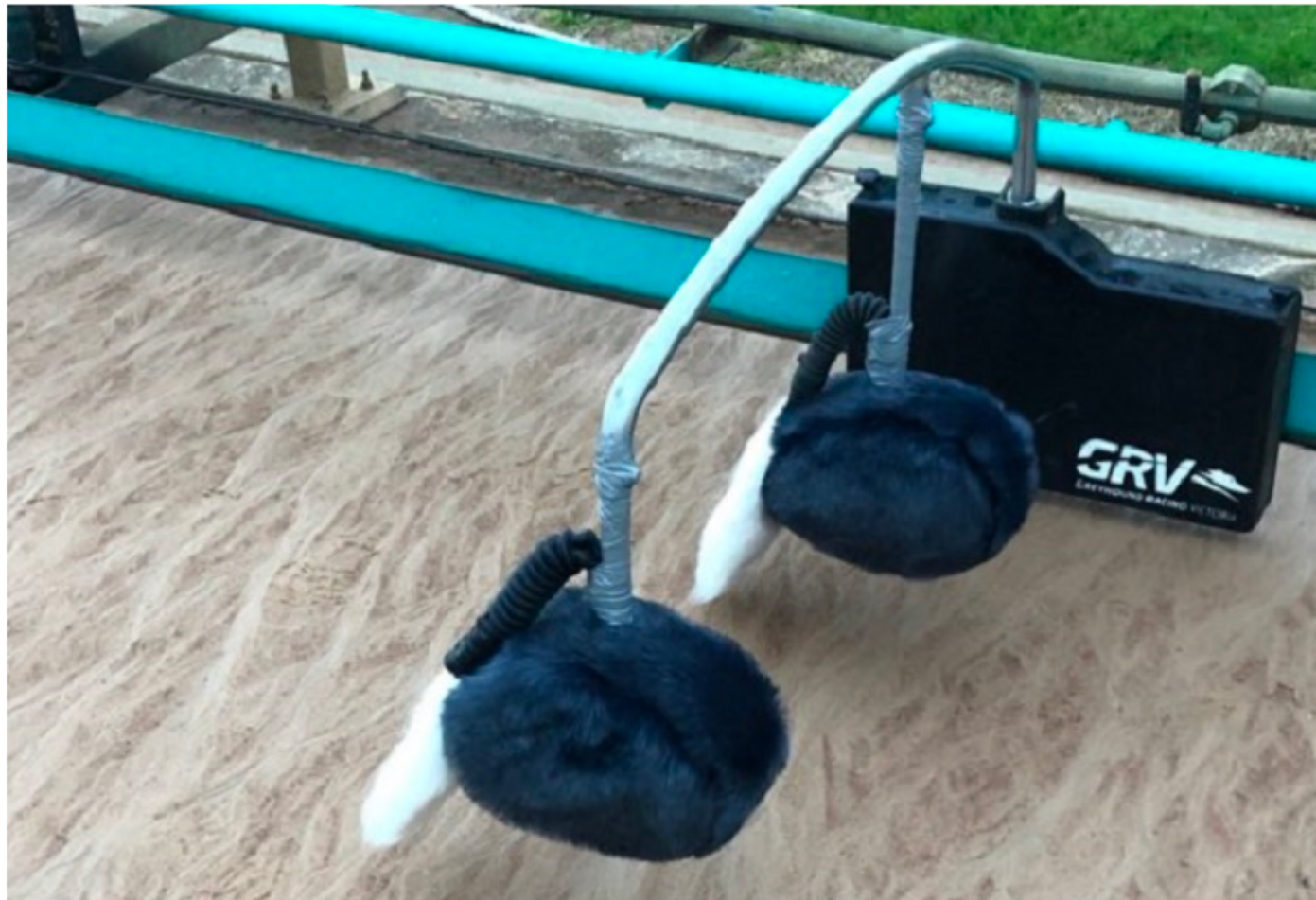
Figure 3: Lure 3 – The lures were located 500 mm and 1200 mm horizontally from the inner rail. In the vertical plane they were 200 mm (lowest distance) and 350 mm (highest distance) above the ground.
