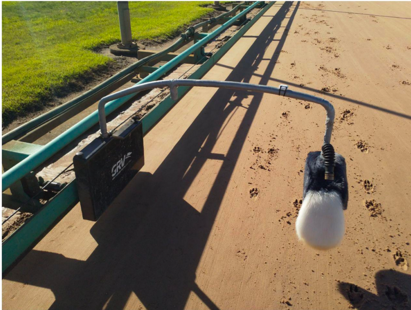
Figure 2: Lure 2 – The lure was located 1200 mm horizontally from the inner rail. In the vertical plane it was 200 mm (lowest distance) and 350 mm (highest distance) above the ground.
