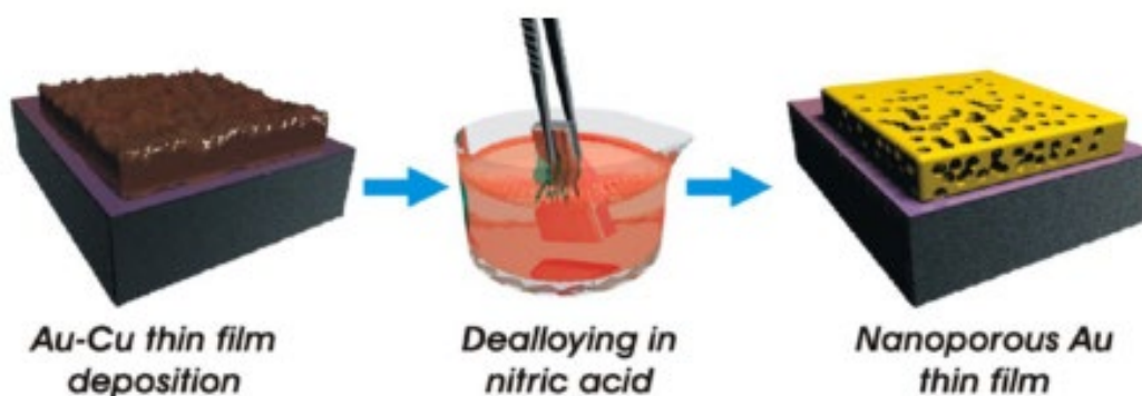
Figure 2 Outline of general steps taken to produce nanoporous metallic sponges from precursor alloys 10 .
