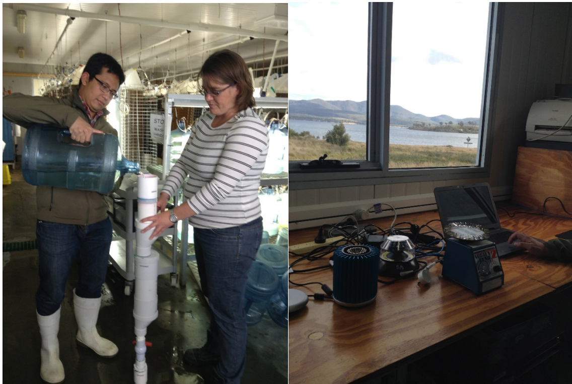
Figure 5. 1. The Phytoxigene™ DinoDtec pipeline filtration system (left), and on-site qPCR set up (right)
