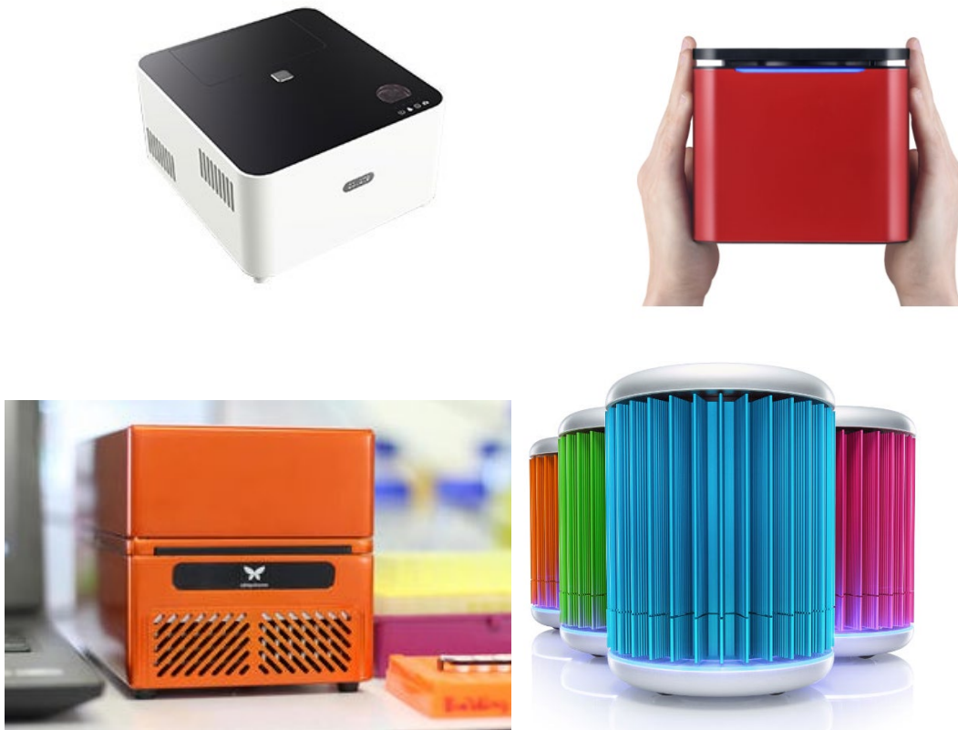
Figure 1. 4. Portable qPCR platforms from various manufacturers, suitable for lab or on-field application (From upper left to right: Mini8 (Coyote Bioscience USA Inc), Mic (Bio Molecular Systems), Liberty16 (Ubiquitome Limited), MyGoMini (IT-IS Life Science)
