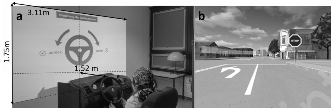
Figure 1: a) Driving simulator setup and b) the previously used hologram arrow projected into the virtual environment (Figure adapted from Wunderlich & Gramann, 2018).
