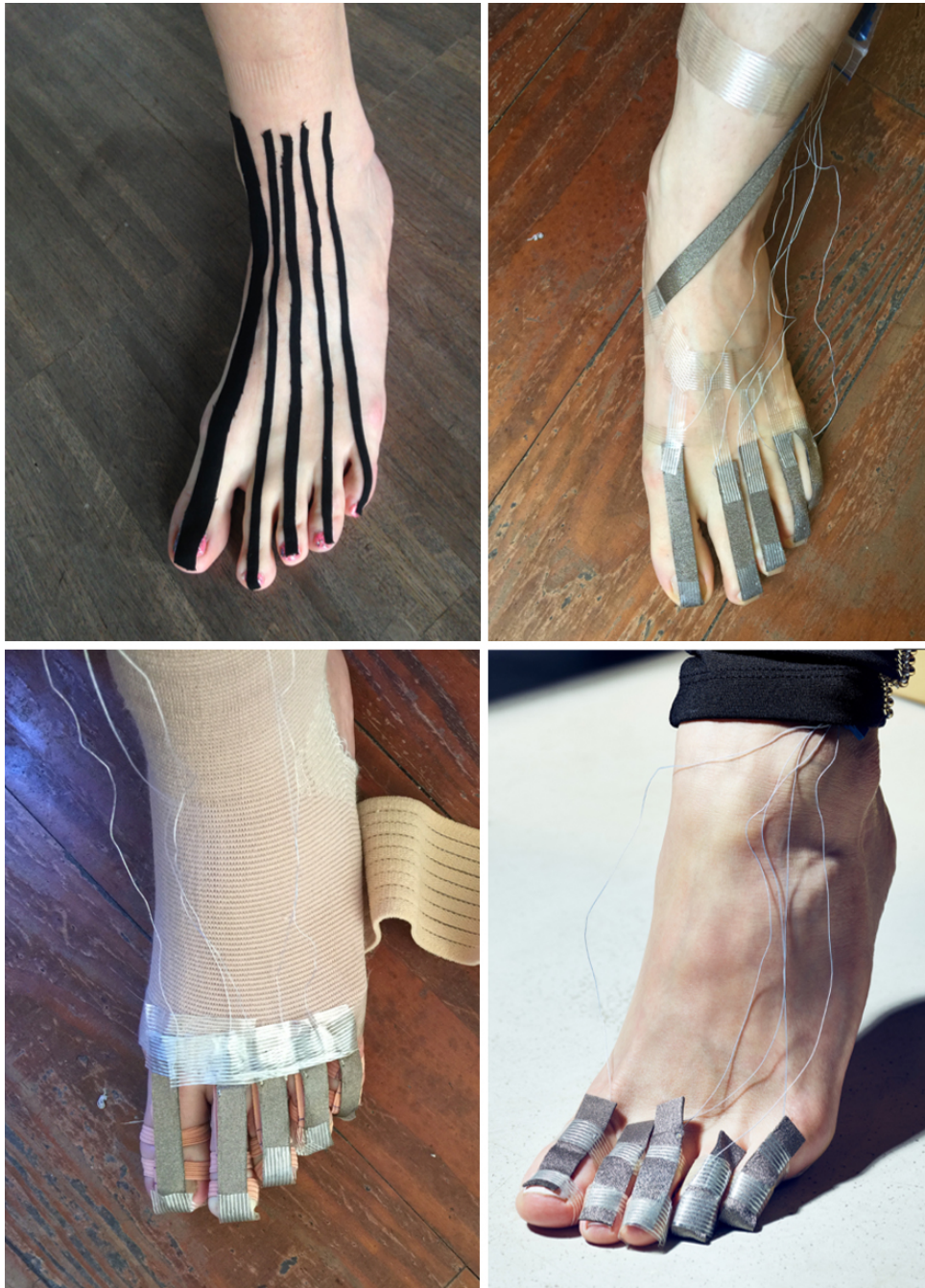
Figure 126. Iterations of attaching toe sensors to the feet. Top left: mock ups with kinesio tape. Top right: medical tape and StretchSense sensors. Bottom left: plantar fasciitis compression foot sock, medical tape and StretchSense sensors. Bottom right: Stretchesense sensors attached to the toes with medical tape.
