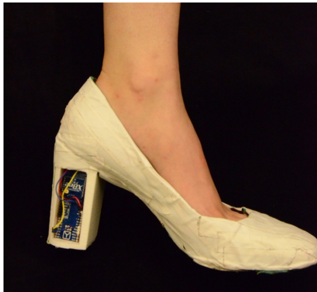
Figure 63. Original Bruno Magli shoe upper covered with duct tape, with 3D-printed heel, Arduino Uno circuit and minimum 9 V3.
