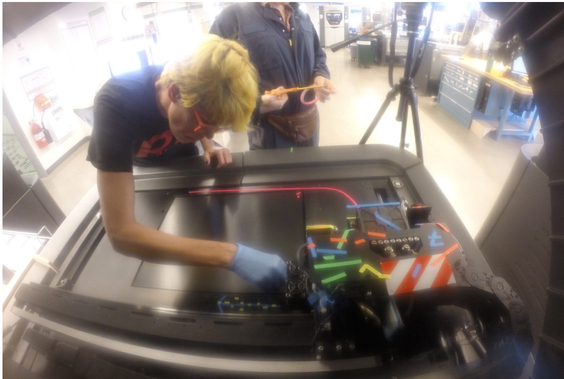
Figure 103. In-laying strips of Mylar film during 3D printing process.
