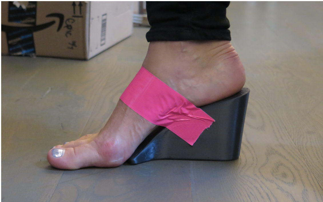
Figure 100. Low resolution 3D printed foot wedge for checking foot bed, structural stability and aesthetics.
