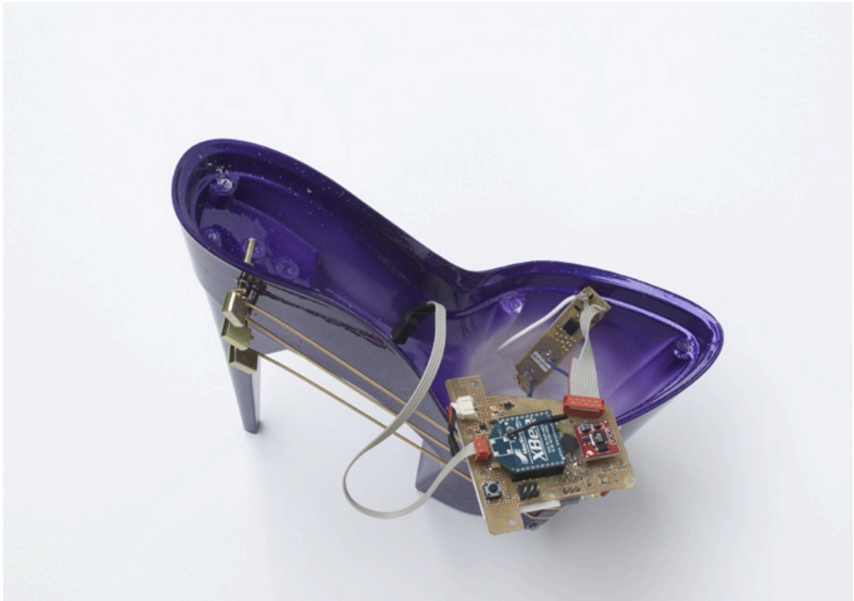
Figure 16. E-Shoe open plateau with bespoke circuit, sensors and XBee transmitter 2011.
