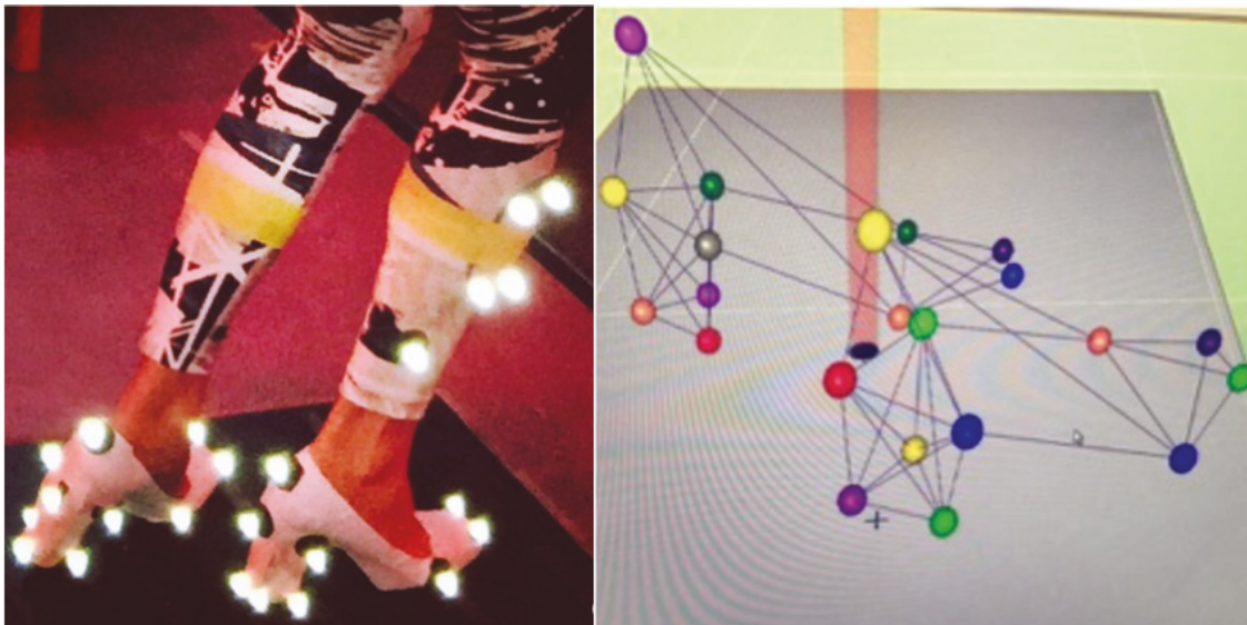
Figure 66. Infrared points attached to key points of CEF P1 high-heeled shoes and shins to analyse movement in 3D motion data acquisition for the Biomechanical Analysis of 3D motion capture data.
