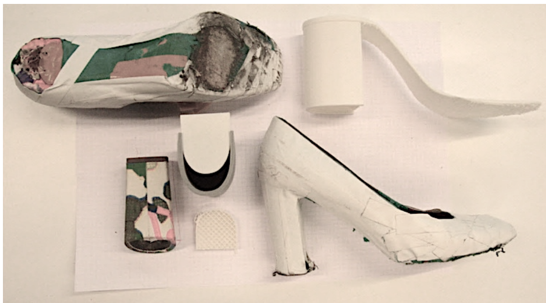
Figure 62. Top Left: Original Bruno Magli high-heeled shoe. Below left: detached heel. Top Right: first 3D-printed prototype shoe. Bottom Right: Original Bruno Magli Shoe covered with white duct tape.
