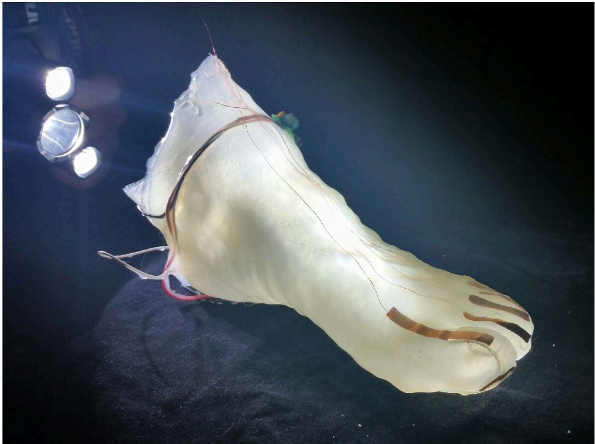
Figure 130. Silicone foot sock with embedded copper strips (to emulate the toe stretch sensors).
