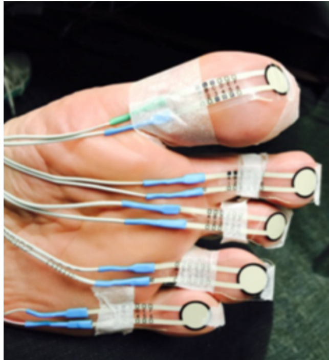
Figure 70. Wired pressure sensors (attached to portable data acquisition system) on the sole of the foot to measure contact of the toes with the ground.
