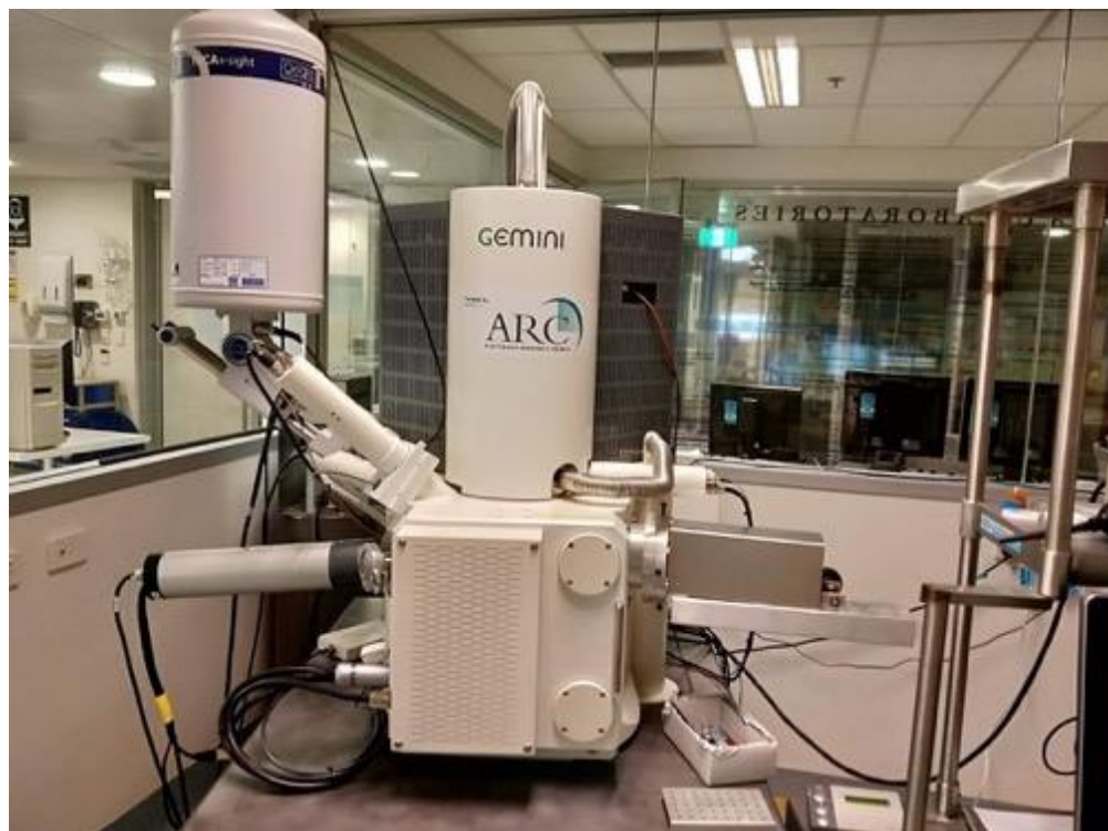
Figure 2.3 – The SEM used to investigate the structural features and morphology of the deposited samples
