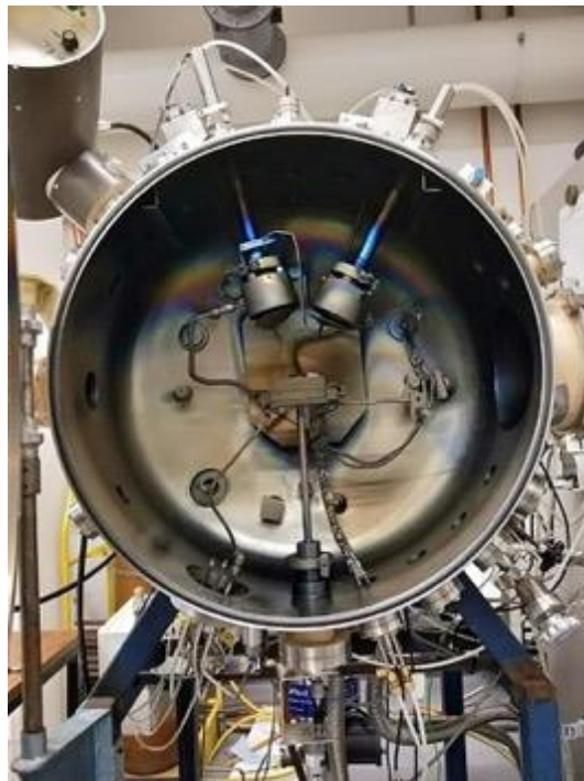
Figure 2.1 – a) A schematic of magnetron sputtering system using Al target as an example; b) a dual target magnetron sputter used to deposit the coatings for CSP
