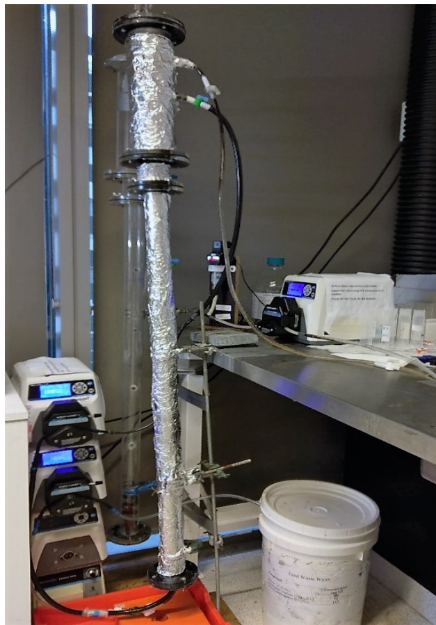
Figure 3.2: AnMBR setup for the production of VFA
