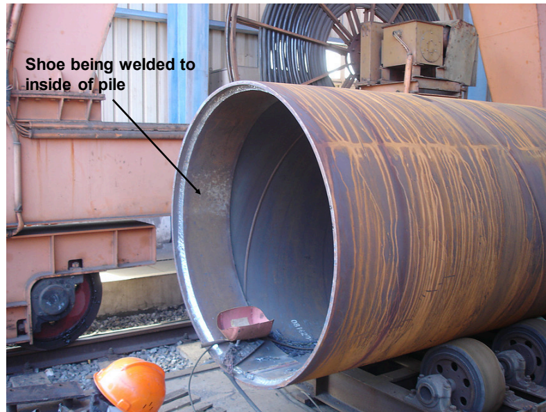
Figure 2.4 Driving shoe, which is welded at the pile toe (ESC Group 2018)
