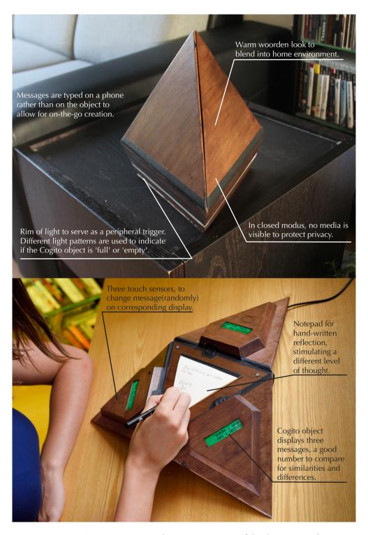
Figure 7.7 Cogito prototype with important aspects of the design rationale.
