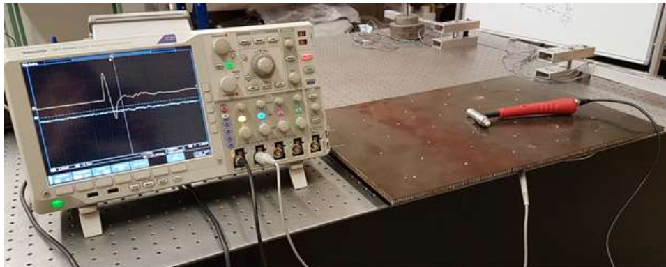
Figure 1. The experimental set-up including the composite panel, impact hammer, oscilloscope, and PZT disk.
