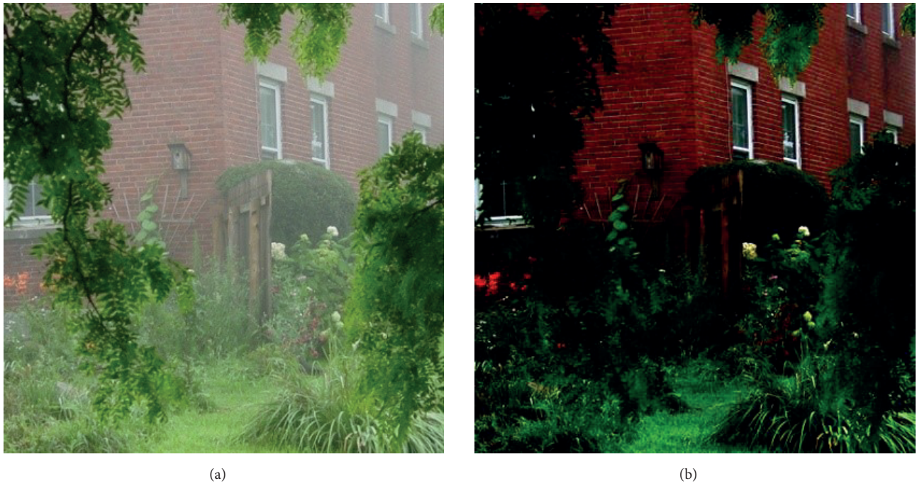
Figure 6. a) Haze image, b) haze-free image using transmission map estimation based on a fuzzy inference system.
