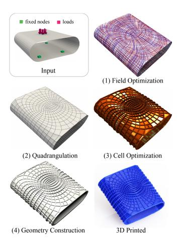
Fig. 1. Stages of our shell structure generation pipeline.
