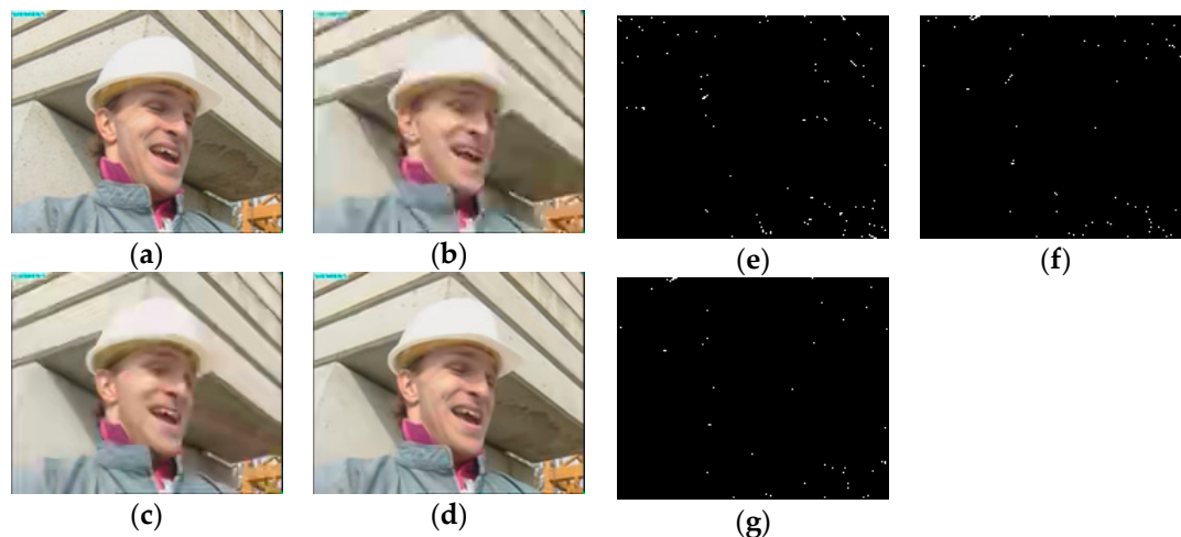
Figure 8. Evaluation of visual quality consistency for the 14 th decoded key frame of Foreman sequence obtained by (a) Original, (b) DISCOVER DVC, (c) H.265-DVC, and (d) proposed JEM-DVC. The bottom row shows the distortion images between the decoded key frames and the original frame, obtained by (e) DISCOVER DVC, (f) H.265-DVC, and (g) proposed JEM-DVC.
