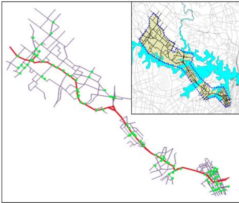
1 2 Figure 2. Victoria corridor sub-network. Green points show signals equipped with SCATS 3 count detectors (measured traffic data). Red line demonstrates the main Victoria corridor.
