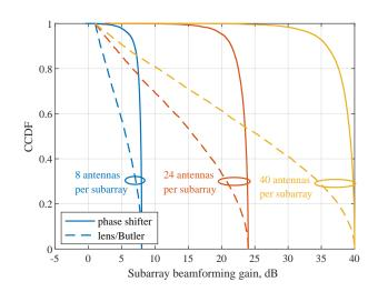
Fig. 6. CCDF of subarray gain based on the AoA estimates in Fig. 5.
