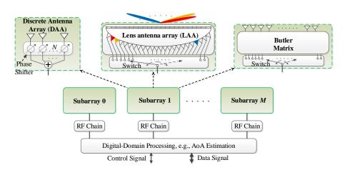
Fig. 2. Schematic diagram of a one-dimensional localized hybrid array, where the subarrays can be implemented by either generic discrete antenna elements, or highly integrated antennas such as lens and Butler matrix.
