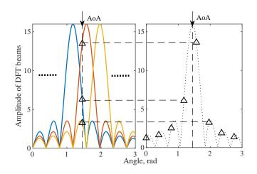
Fig. 3. Illustration of the amplitudes of consecutive DFT beams and the responses of the DFT beams at the target AoA.
