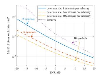
Fig. 5. MSE of AoA estimation vs the received SNR at antennas, where the new AoA estimation approach in Section III; referred to as "deterministic", is compared with the state-of-the-art approach, referred to as "iterative" [9].
