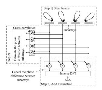
Fig. 4. System diagram of the new unambiguous AoA estimation algorithm developed based on the two new discoveries described in Section III-A.
