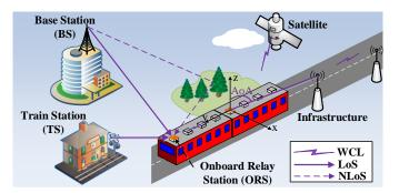
Fig. 1. Schematic diagram of the "smart" railway communication system with the interconnections between the HST and BS, TS, infrastructures, as well as satellite. WCL refers to wireless communication link.
