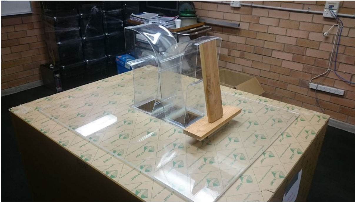
Figure 5-3. Two sided windcatcher fitted on the acrylic chamber
