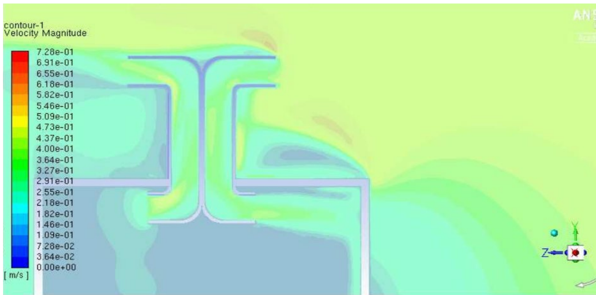
Figure 3-53. Velocity magnitude representation of the room and windcatcher with 0.5 m/s wind speed at the domain's inlet
