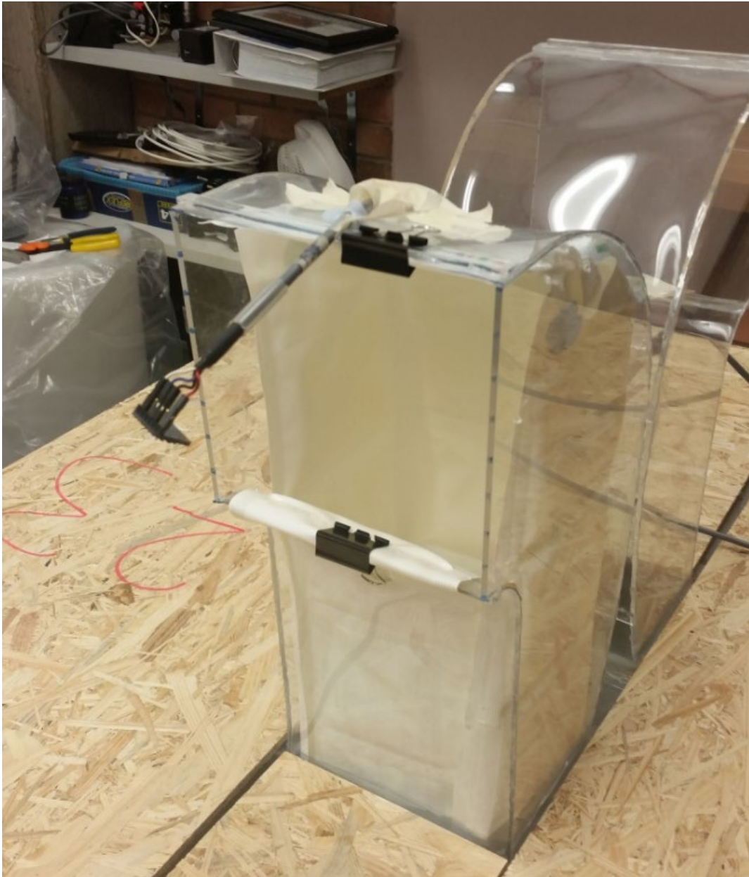
Figure 5-9 PCM placed in the windcatcher's inlet channel
