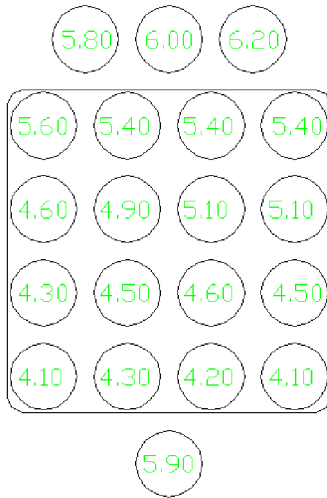
Figure 4-23. Distribution in % of total air flow rate through the module at 2380 RPM fan speed
