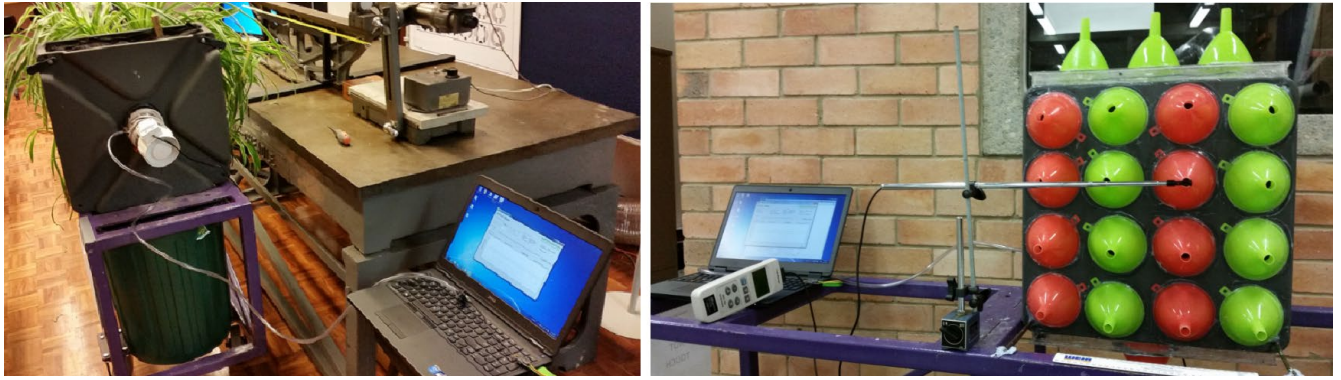
Figure 4-3. Green wall module with funnels attached (16 covering the front openings, 3 on top and 1 at bottom).
