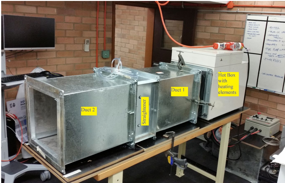
Figure 5-11 Set up for the Hot Box and ducts
