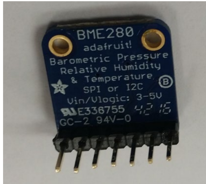
Figure 4-26 Adafruit BME280 Pressure Temperature and humidity sensor
