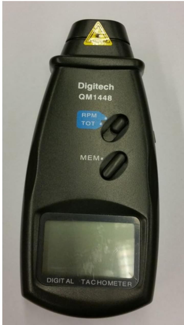
Figure 4-19. Digitech digital Tachometer QM1448
