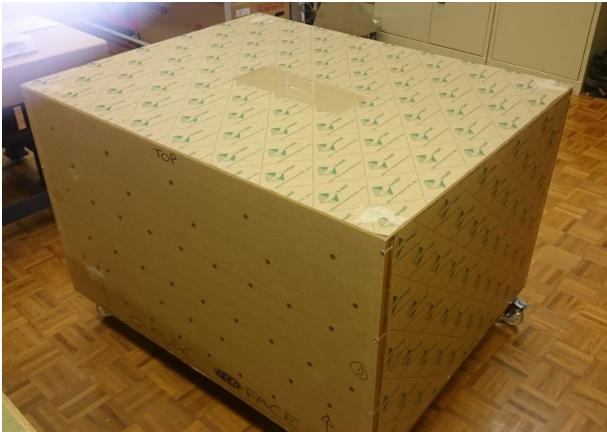
Figure 5-1. 12 mm acrylic sheets chamber (1250 x 1000 x 750 mm 3 ) with wheels.
