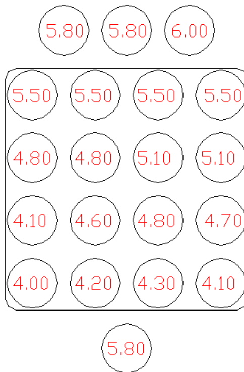
Figure 4-24. Distribution in % of total air flow rate through the module at 2220 RMP fan speed
