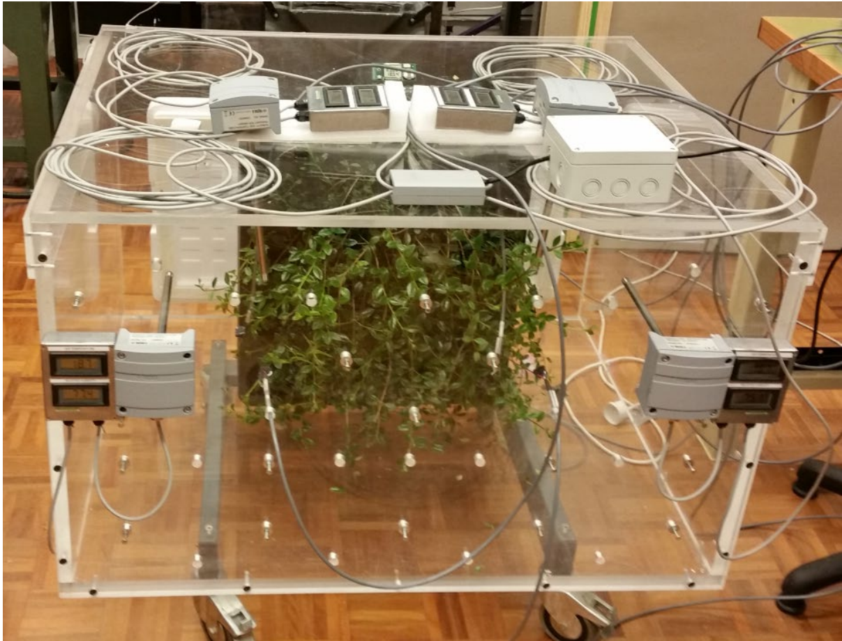
Figure 1-20. Set up to monitor effect of Green Wall module on Temperature and humidity
