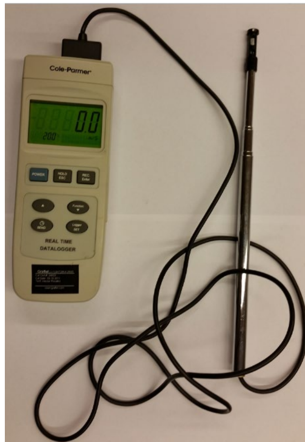
Figure 4-4. Hot wire anemometer used to measure air velocity.
