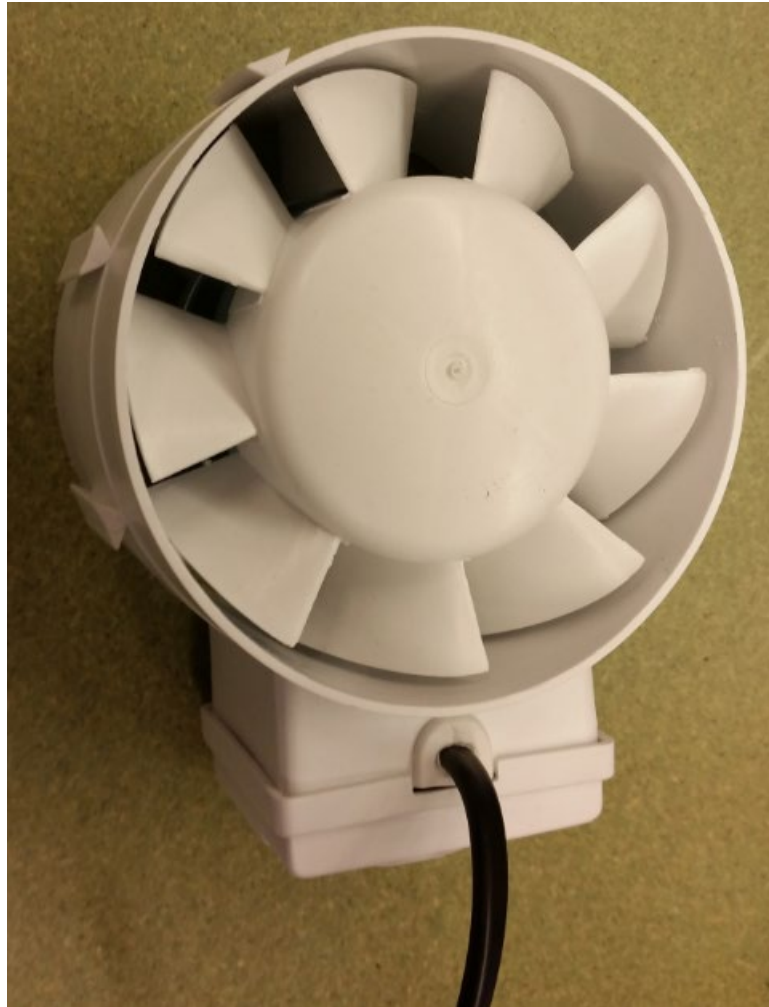
Figure 4-2. A constant-speed FANTECH TEF-100 16-W in-line axial fan
