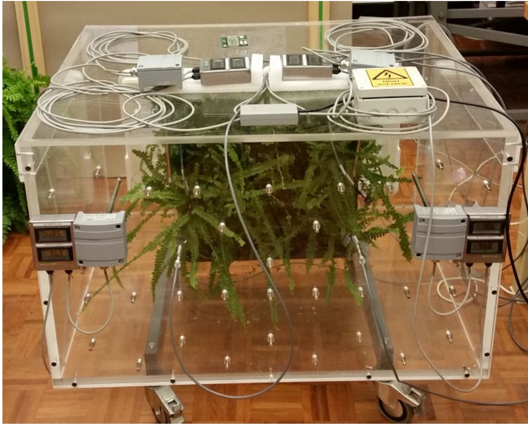
Figure 4-25. Acrylic-sheets chamber with a green wall module ( Nephrolepis cordifolia )
