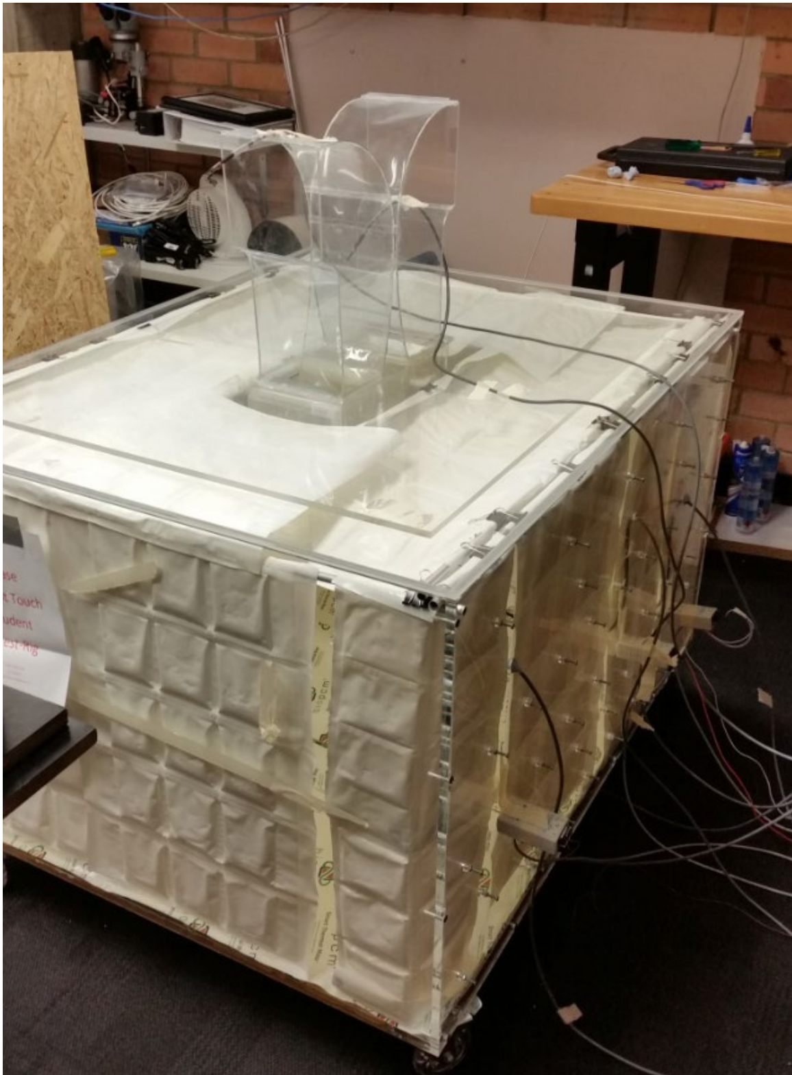
Figure 1-21. PCM placed on floor, walls and ceiling of the room fitted with a windcatcher
