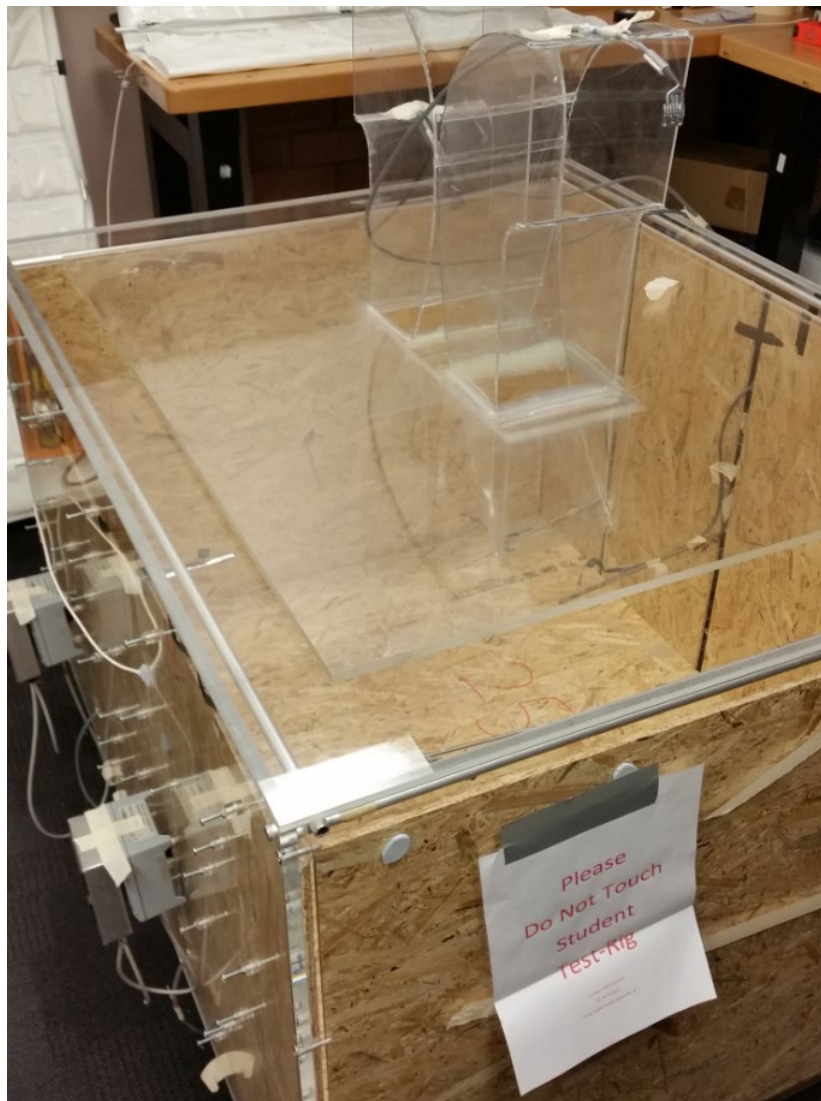
Figure 5-5 Acrylic chamber with plywood placed at the walls and the floor
