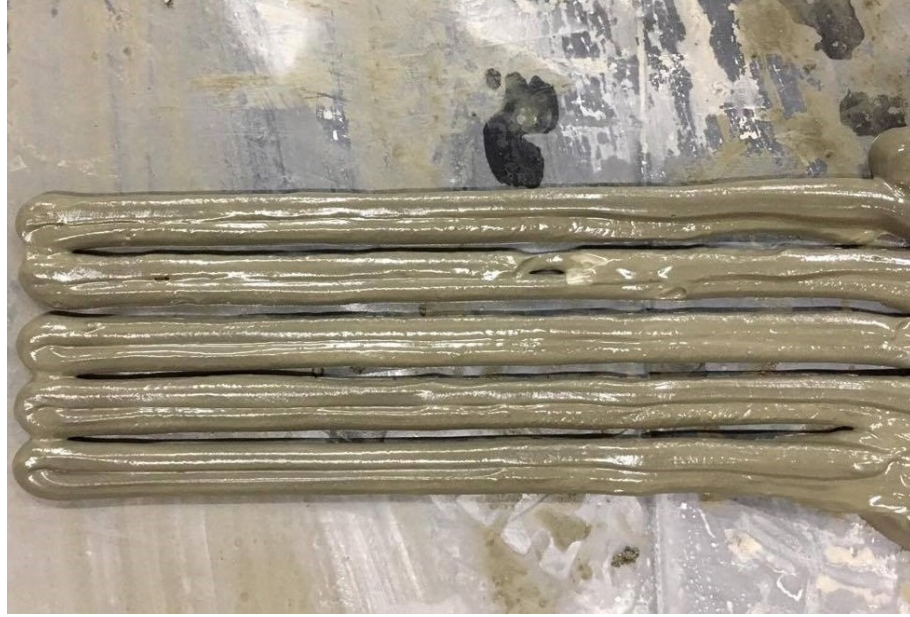
Figure 4. 8: Printed cement mortar using a peristaltic pump with a 7.9mm diameter.
