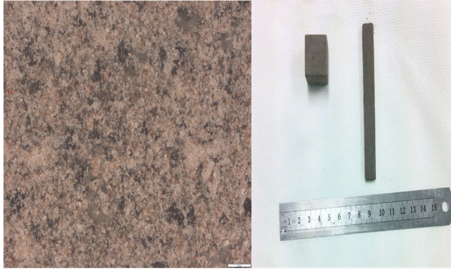
Figure 5. 11: Morphology surface of cubic specimens (left) (Olympus BX61 Microscope-10×) and samples of CAC, OPC with \text{Li}_2\text{CO}_3 prepared by 3D printing (right).
