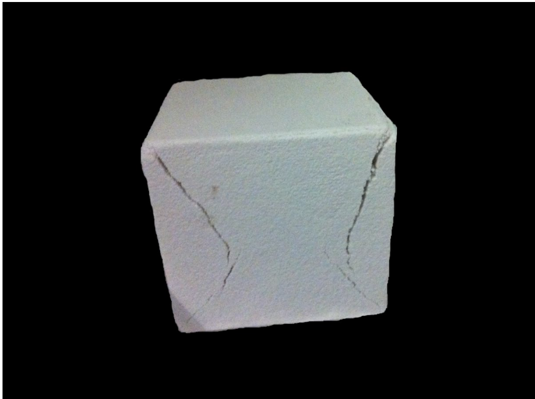
Figure 6. 3:(50 × 50) mm diagonal crack inside the Z-powder specimen.
