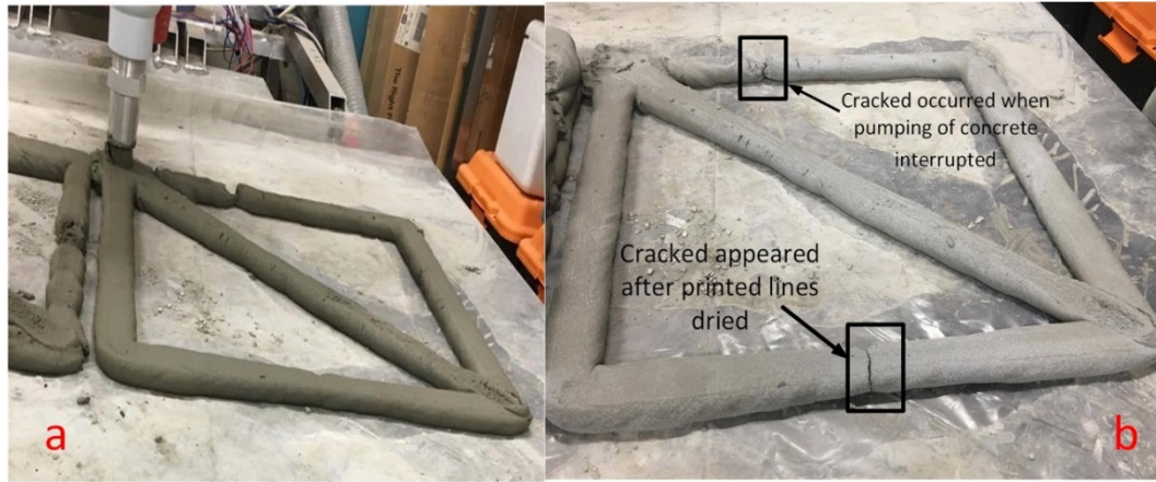
Figure 3. 5: (a) Printed mortar via extrusion printing, (b) Printed mortar using robot extrusion dried in ambient temperature for one day.
