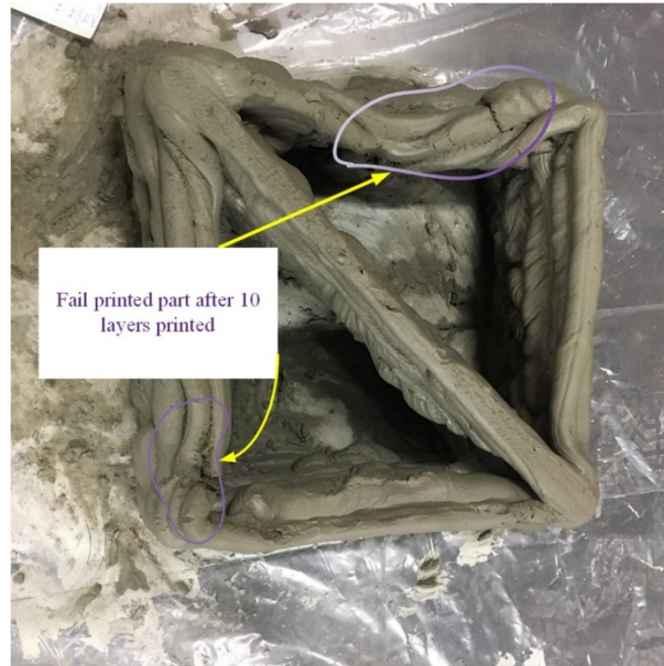
Figure 5. 34: The movement of the robot arm has a major effect on the printing process, particularly when the height of the object increased to more than 7 layers.
