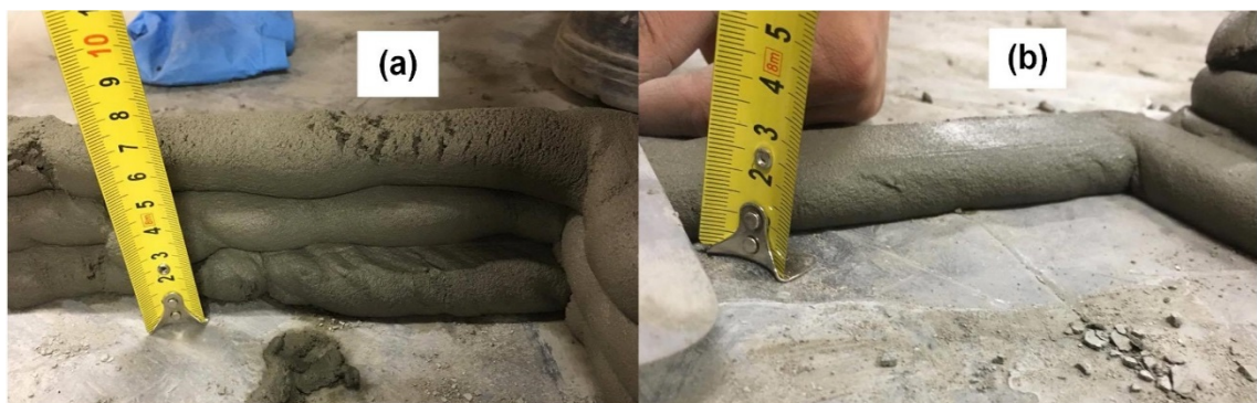
Figure 5. 33: (a) Three layers of the printed object; (b) One layer of the printed object.
