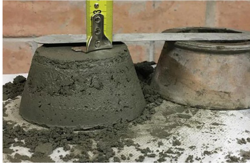
Figure 6. 59: Mini-cone slump test for trial 8.
