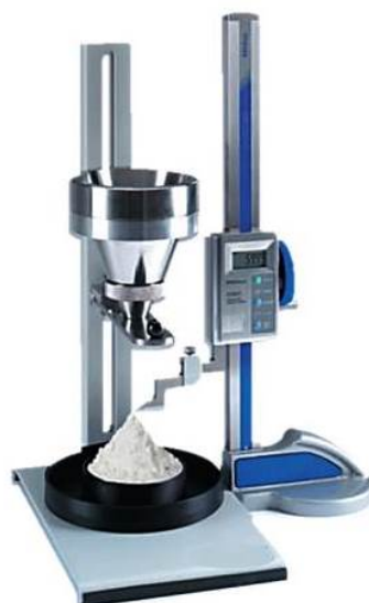
Figure C. 4: Powder flow test apparatus
