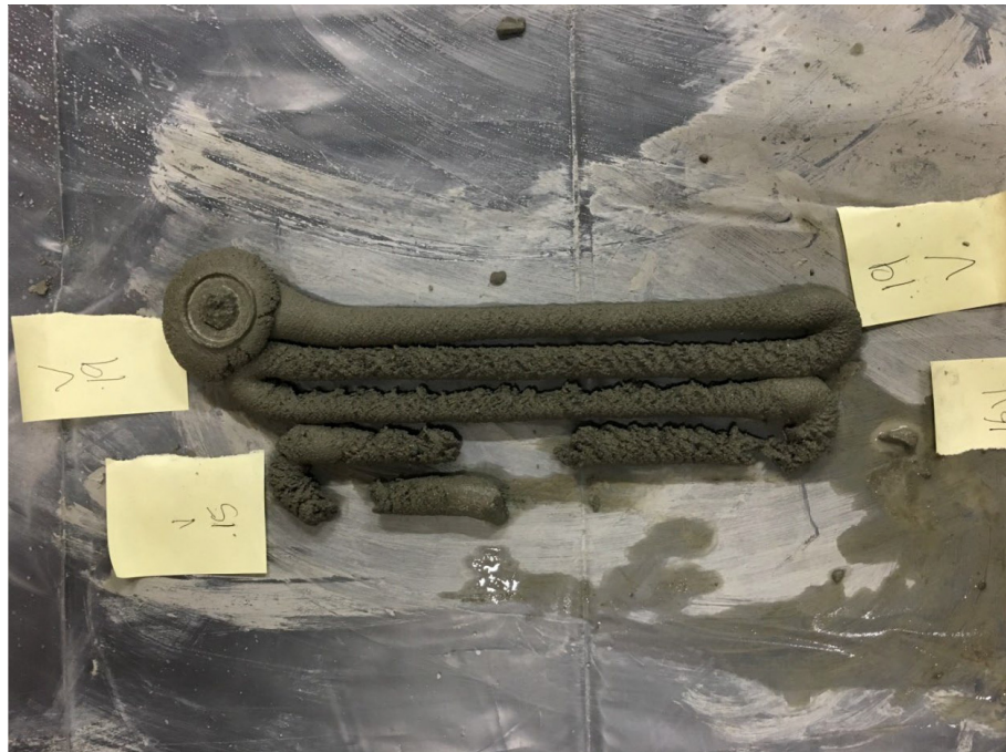
Figure 4. 6: Resultant Print of successful print yielding a stable mortar and decent slump slurry. Issues with the auger delivery struggling to consistently push out materials.
