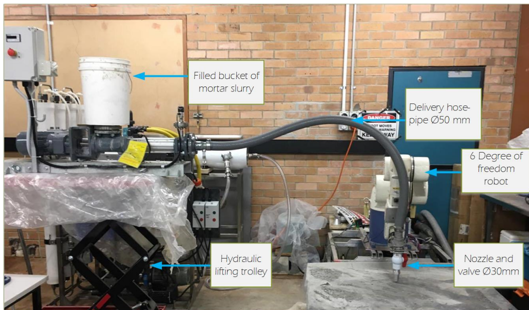
Figure 5. 28: The final system with the progress cavity pump connected to the robot.
