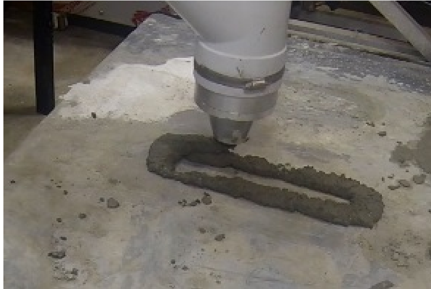
Figure 3. 1: Printed concrete through a custom-made delivery system (note: a max. particle size of coarse aggregate of approximately 5mm)
