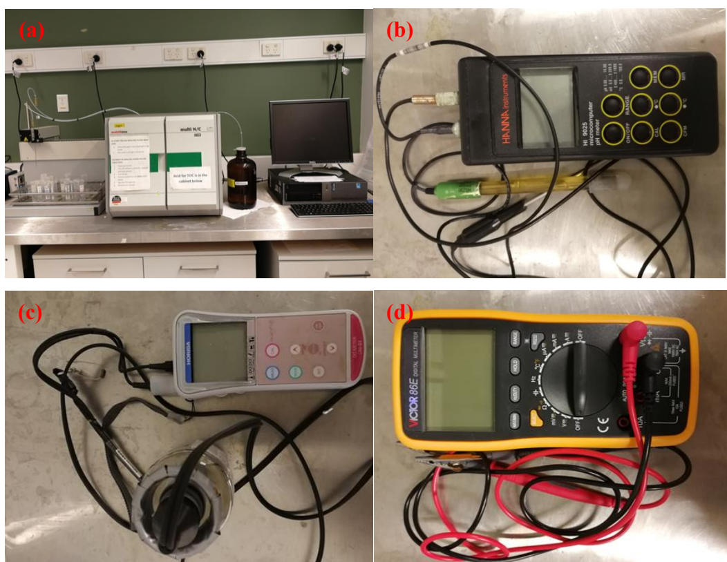
Figure 3.3 The analytical instruments used in the experimental investigation: a) TOC analyser; b) pH meter; c) DO meter; d) universal digital meter
