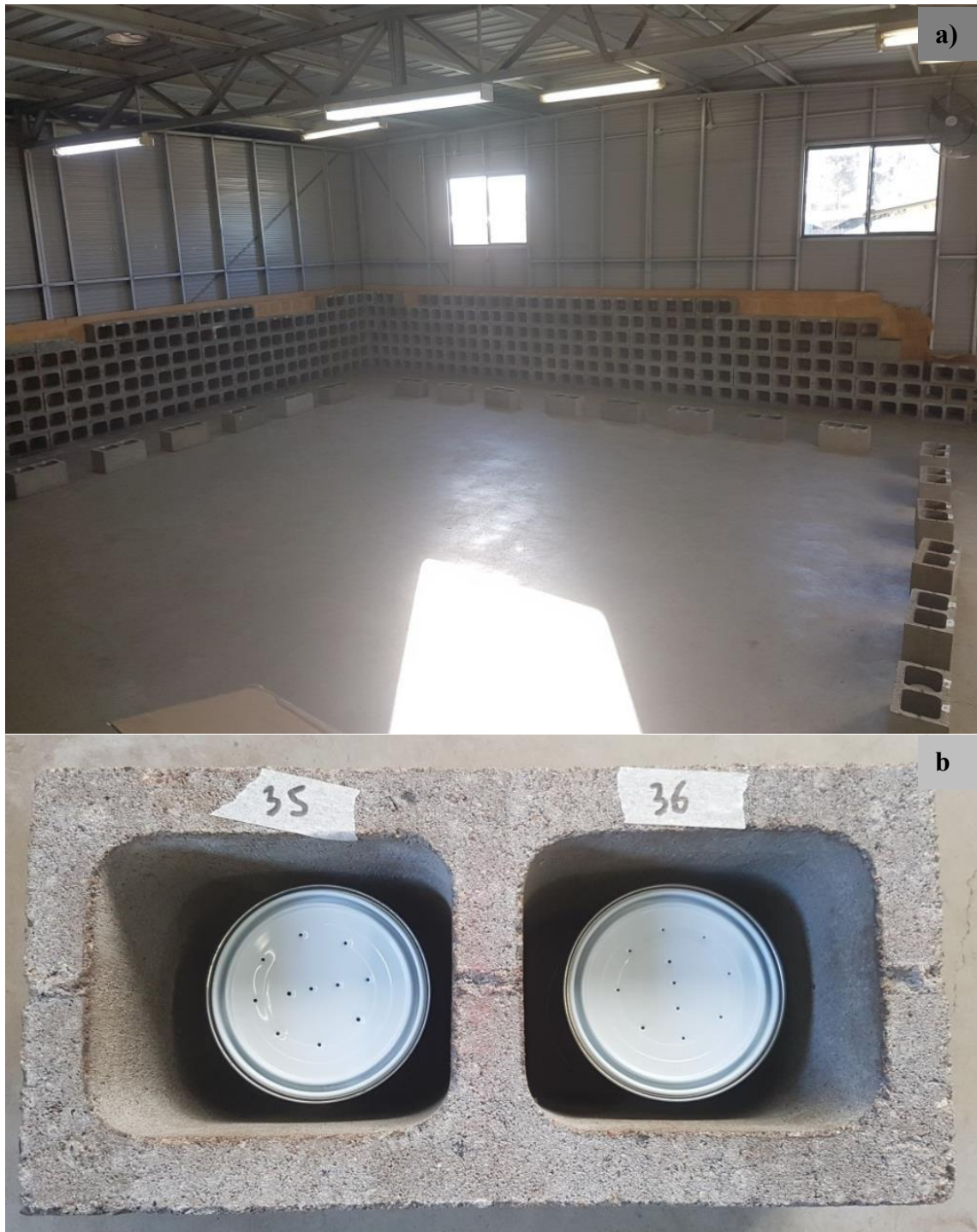
Figure 5-2: Scent line-up and sample placement; a) shows the room configuration and b) the perforated aluminium tins contained within each cinder block. Figures adapted with permission from Rust, 2018 [270].
