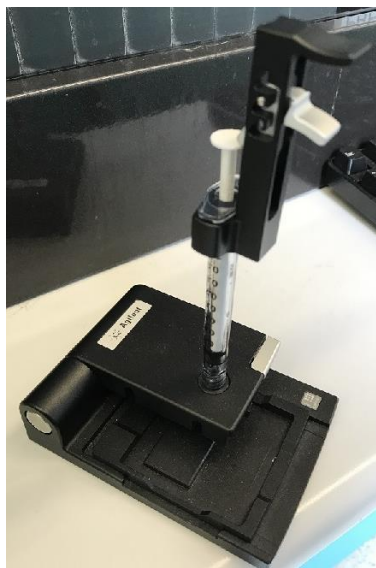
Figure 3-3: Agilent Priming Station used to apply air pressure to the wells of the microchip when priming it.
