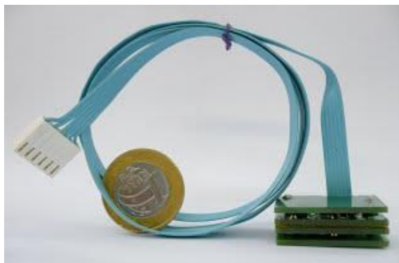
Figure 2-1: Size comparison of a C 4 D system and a Brazilian Real coin. Figure adapted from da Silva et al. , 1998 [167].
