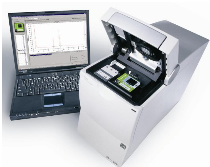
Figure 3-1: The Agilent Bioanalyzer 2100 instrument and laptop for data collection and analysis.
