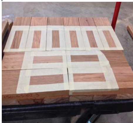
Figure 3-8 Manufacturing of timber joints
