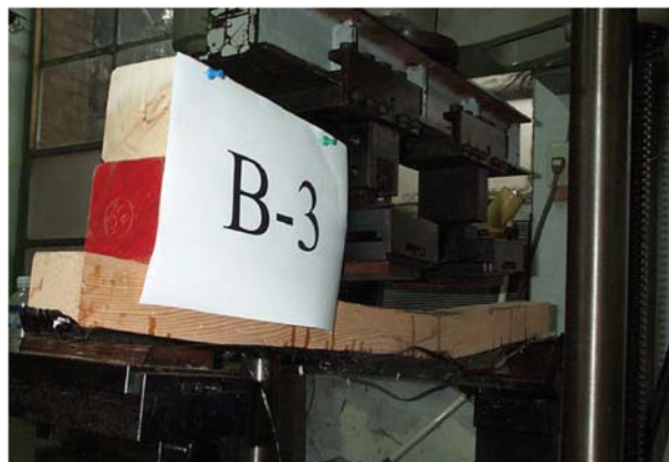
Figure 2-11 Failure mode of the retrofitted timber beams with 1 layer of CFRP sheet (Yang et al. 2008)
