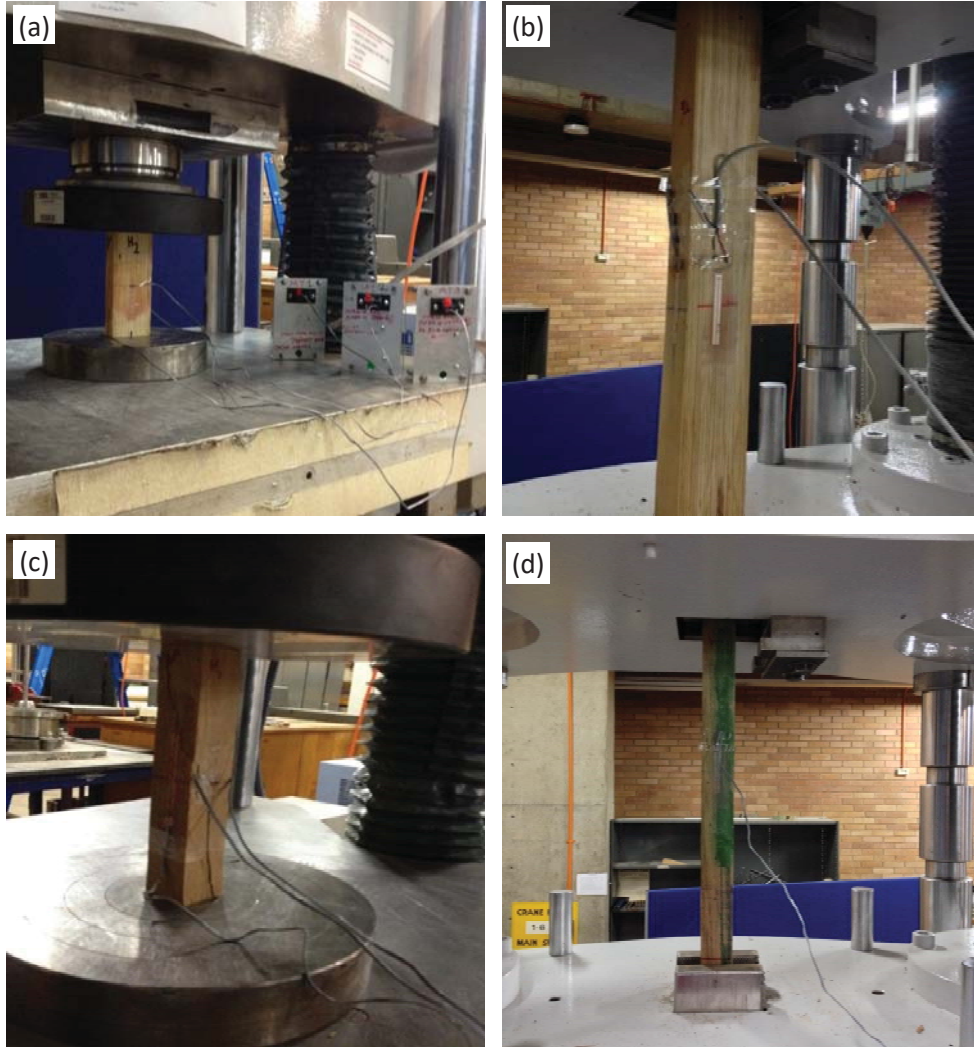
Figure 3-2 Timber specimen test in progress; (a) compressive test of LVL, (b) tensile test of LVL, (c) compressive test of Hardwood, (d) tensile test of Hardwood
