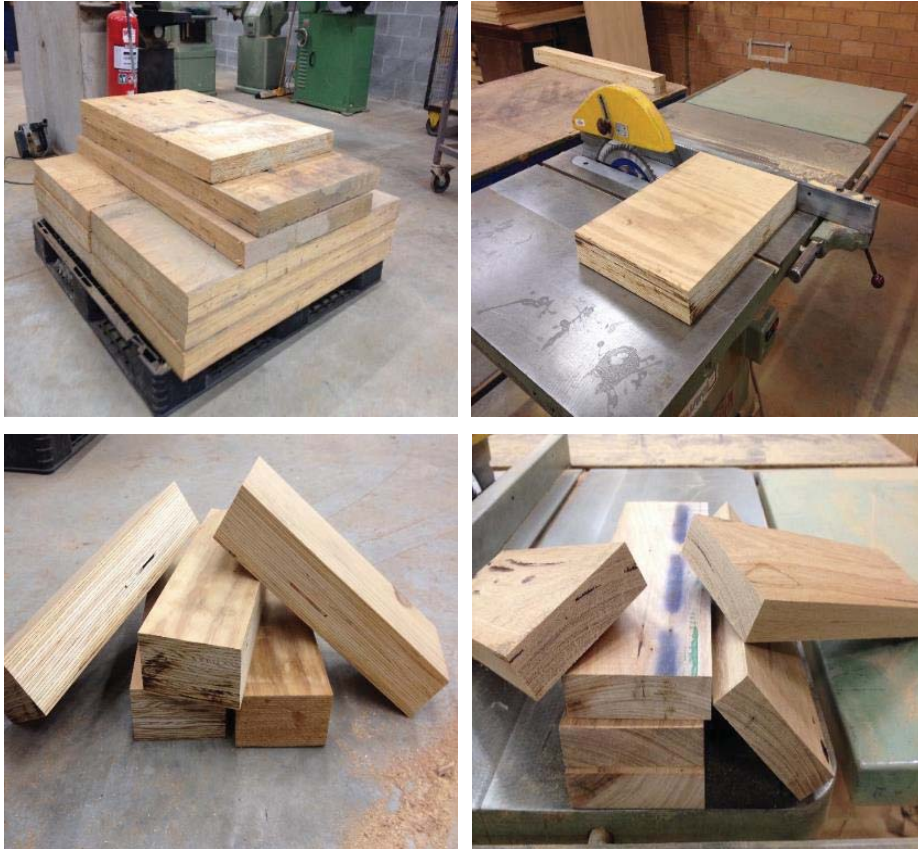
Figure 3-6 Cutting of the timber specimens.
