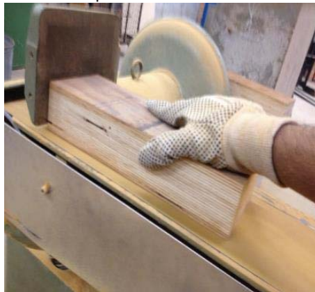
Figure 3-7 Surface preparation of timber block
