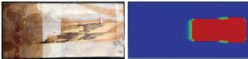
Figure 5-11 Comparison between failure of experimental and numerical result for sample 150-35-02
