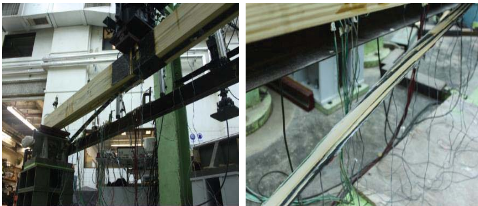
Figure 2-12 failure modes, failed beam and debonded FRP (Wan 2014)
