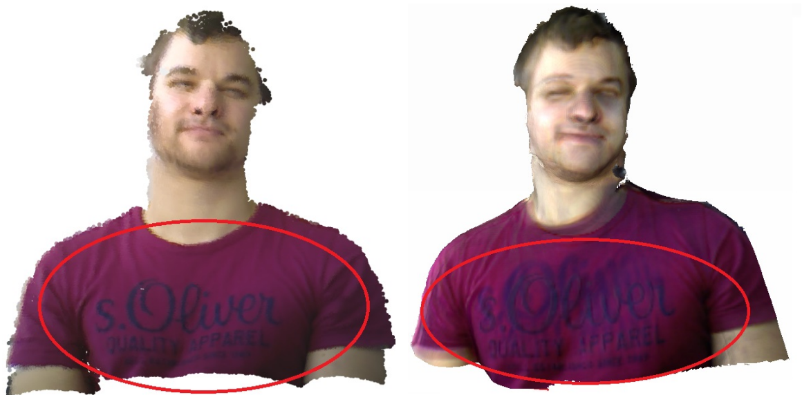
FIGURE 3.13: Comparison with VolumeDeform approach. Left is the result of the robotic template free SLAM. The right is VolumeDeform's result. Note the difference in texture (letters on the T-shirt).
