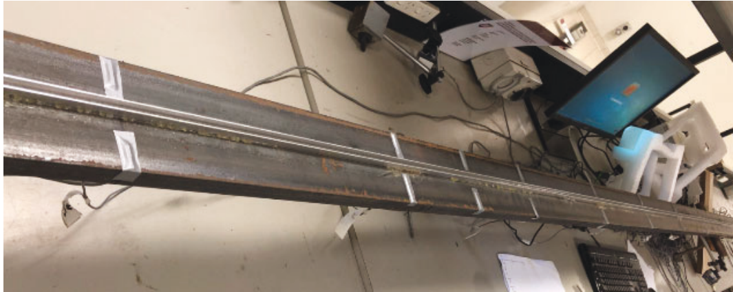
Figure 7.8 The installation of plastic strip to simulate bumps on the bridge
