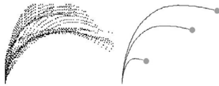
Fig. 7: Paths from training data sharing a similar endpoint orientation are gathered (left); their resulting primitive can then be spatially scaled to arbitrary positions (right, gray circles).
