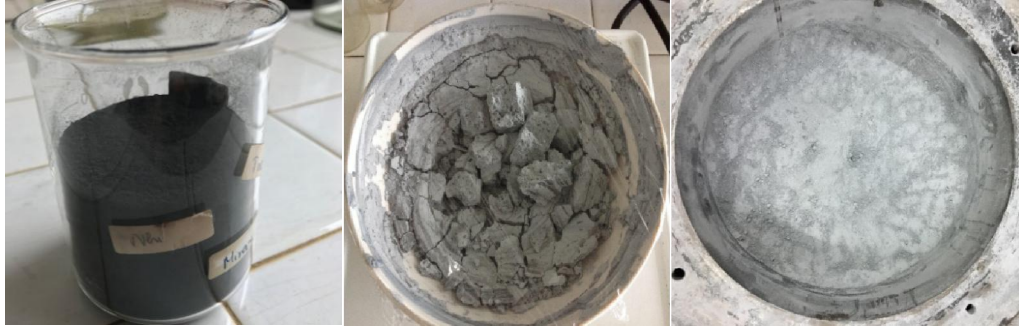
(a) Expanded graphite (b) Dried compound (c) EM8block in the reactor
