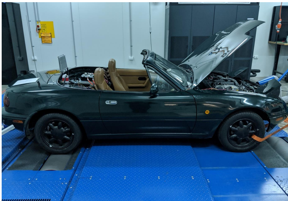
Figure 8.9 Prototype MHEV (KERMIT IV) on the MAHA MSR500/2 dynamometer
