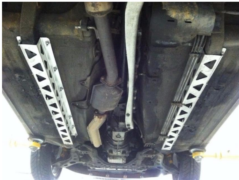
Figure 6.3 Standard MX-5 powertrain showing the PPF connecting front and rear assemblies
