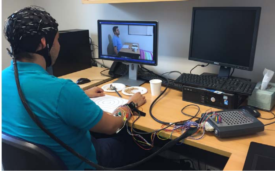
Figure 5-7. Experiment setup for tremor recording
