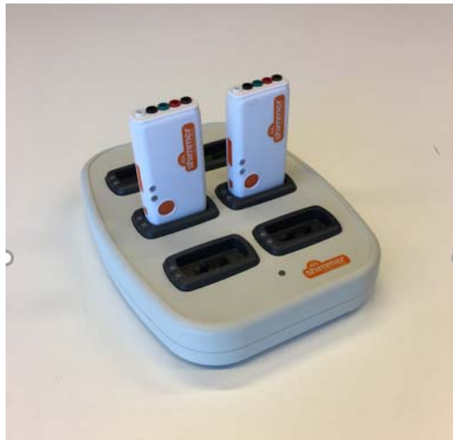
Figure 5-3. IMU used for data recording in the experiment
