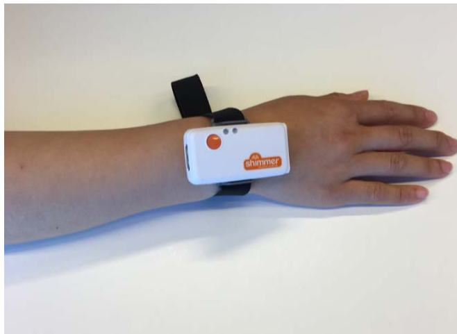
Figure 5-4. The position of IMU attachment on the subject's wrist
