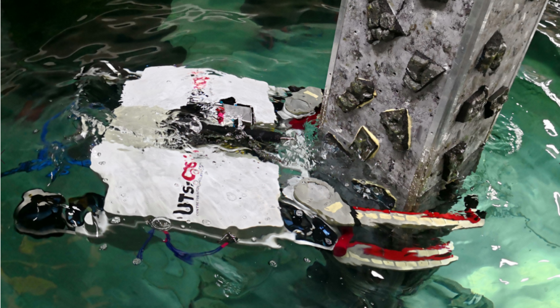
FIGURE 1.3: The SPIR is designed to operate in shallow bathymetry to clean infrastructure.
