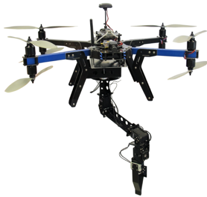
(C) An example of an Unmanned Aerial Vehicle-Manipulator System (UAVMS) (Lunni et al., 2017)
