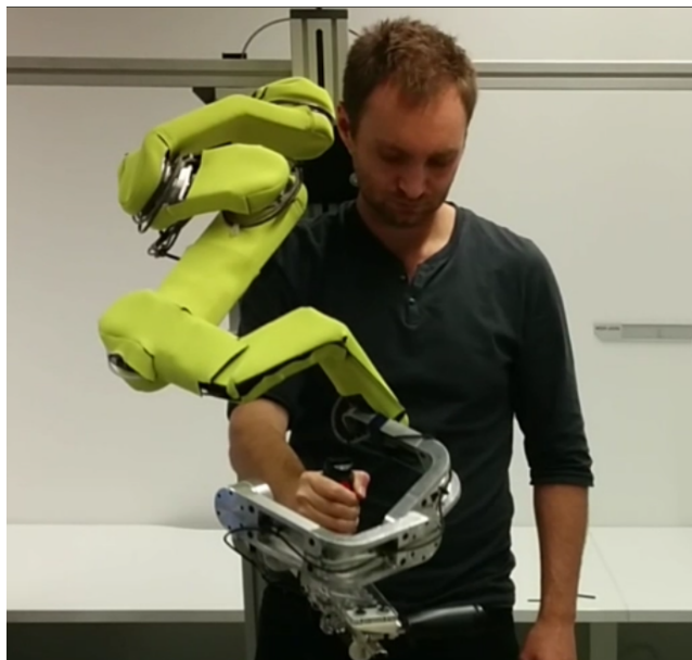
FIGURE 2.4: An upper body exoskeleton the JEXO designed based on the range of motion of the human shoulder to be used in upper limb rehabilitation [6].
