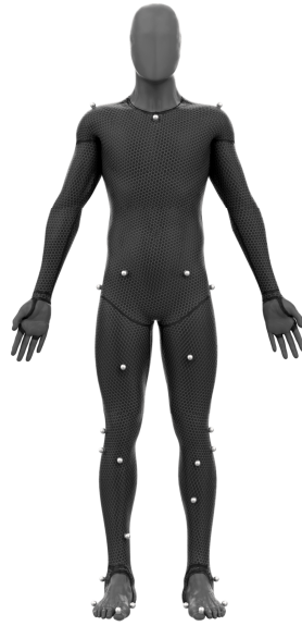
FIGURE 2.5: Motion capture suit worn to track a human using the OptiTrack system [7]
