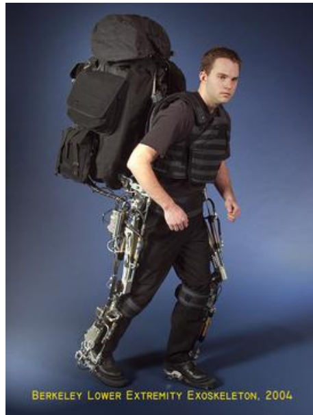
FIGURE 2.3: A human wearing the BLEEX [5] used to support the human carry a heavy load.
