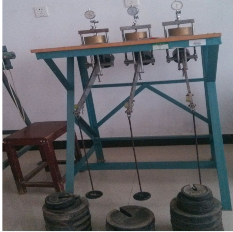
Figure 4.1: Schematic view of consolidation apparatus
