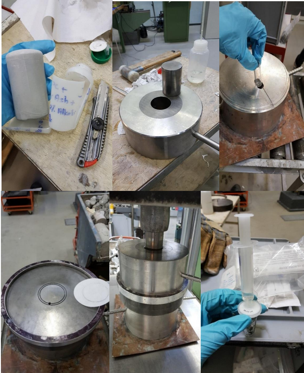
Figure 3-22 Pore solution extraction of blended pastes using 1500 kN force from compression testing machine
