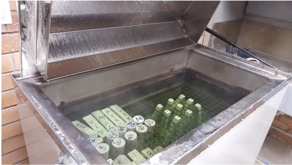
Figure 3-19 1M NaOH bath at 80 °C for accelerating mortar expansion (AMBT)
