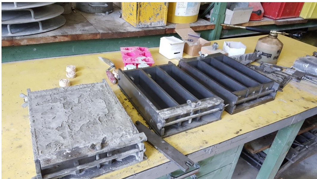
Figure 3-21 Casting of concrete prisms
