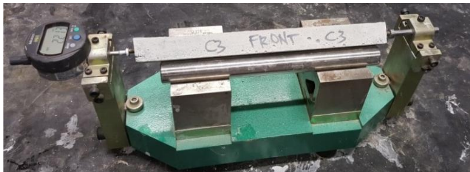
Figure 3-20 AMBT Specimen Expansion Measurement (horizontal comparator)
