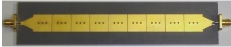
Fig. 4. Top view of a prototype with three vias in a unit cell.
