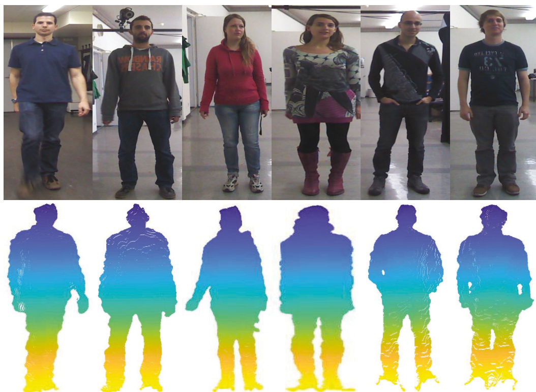
Figure 5.5 : Examples of point clouds. Images in top row is the RGB images in BIWI RGBD-ID dataset and images in bottom row are their corresponding visualization of point clouds.
