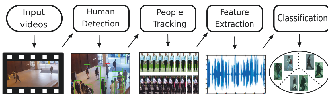
Figure 1.3 : Pipeline of a complete person Re-ID system
