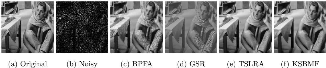
Figure 4.4 : Visual comparison for random missing pixel filling on Barbara. (a) Original image. (b) Image with 20% random samples. (c) BPFA (PSNR=22.30 dB). (d) GSR (PSNR=22.66dB). (e) TSLRA (PSNR=25.34 dB). (f) KSBMF (PSNR= 25.73 dB).
