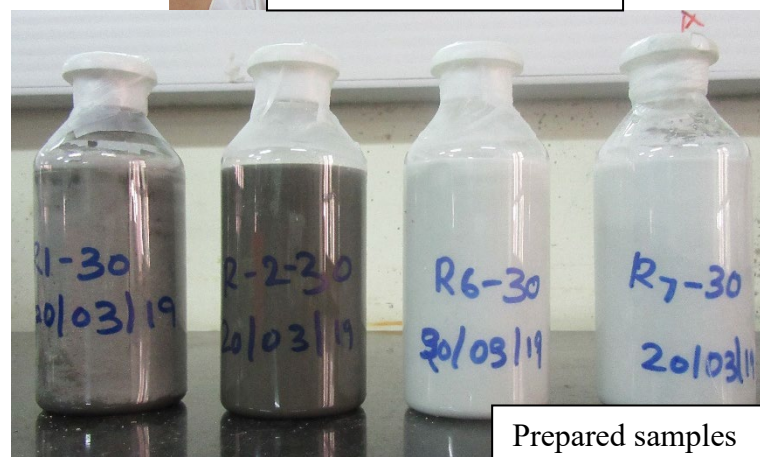
Figure 4.13 Cement paste preparation for pore solution extraction
