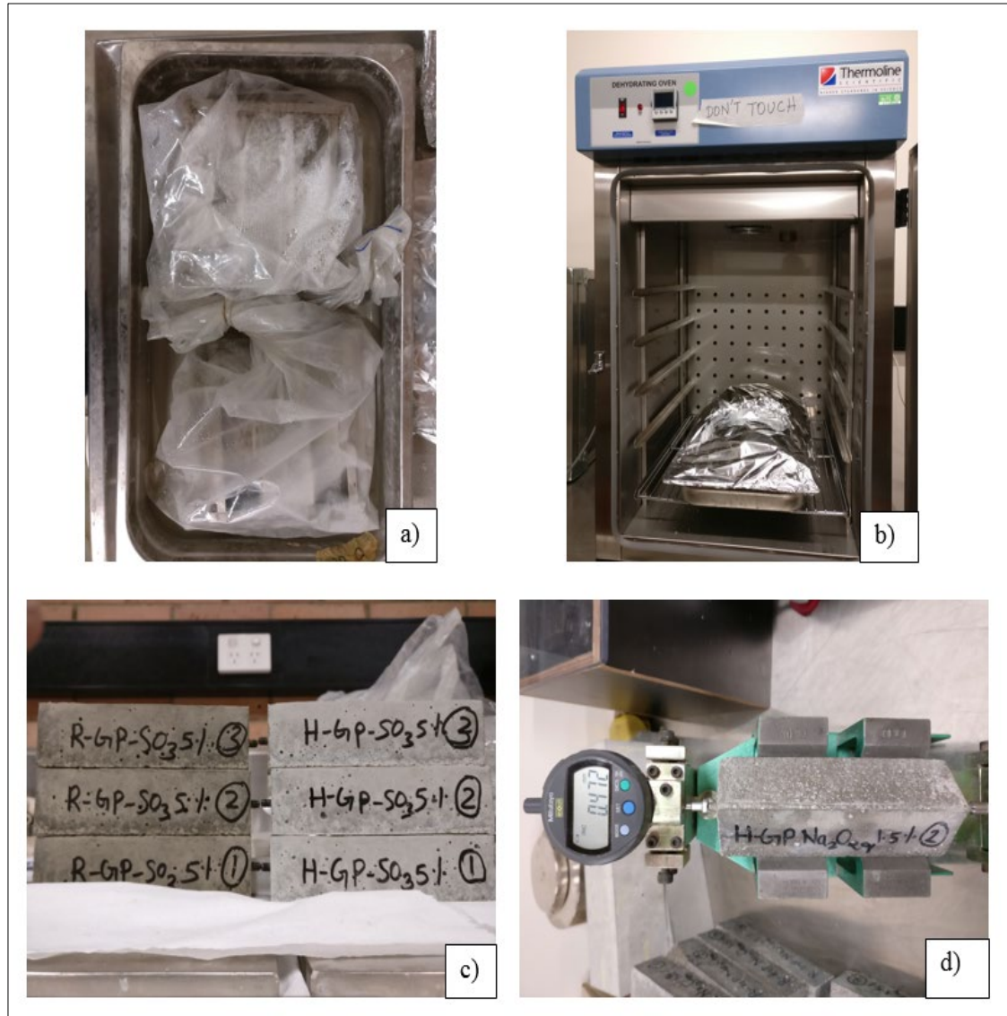
Figure 4.4 a) Water bath containing mortar prisms in sealed oven bag b) Foil covered enclosed system inside oven c) demoulded samples cured in a humidity chamber (left) and oven (right) d) Specimen linear expansion measurement using digital length comparator
