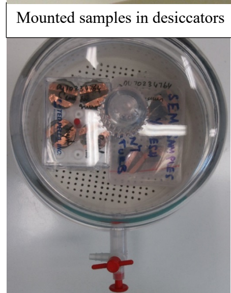
Figure 4.19 SEM sample preparation: Polishing, Au-Pd coating and storage
