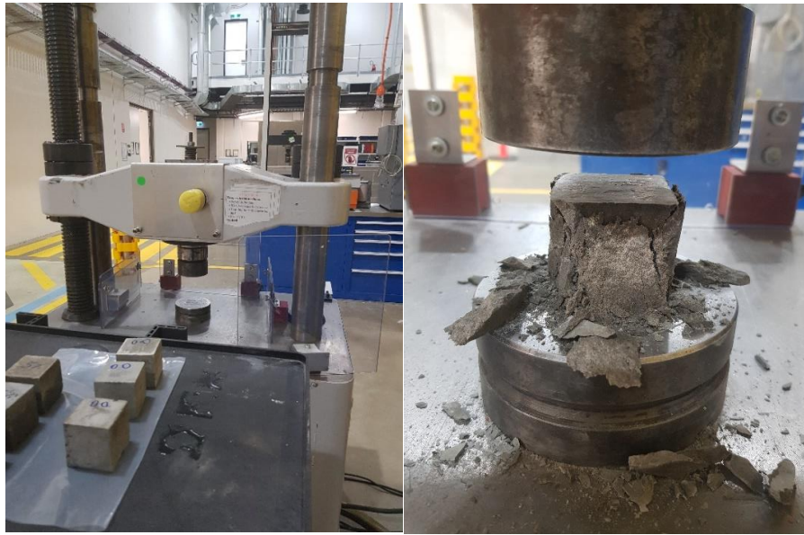
Figure 14. Compressive strength test applied on cement paste.
