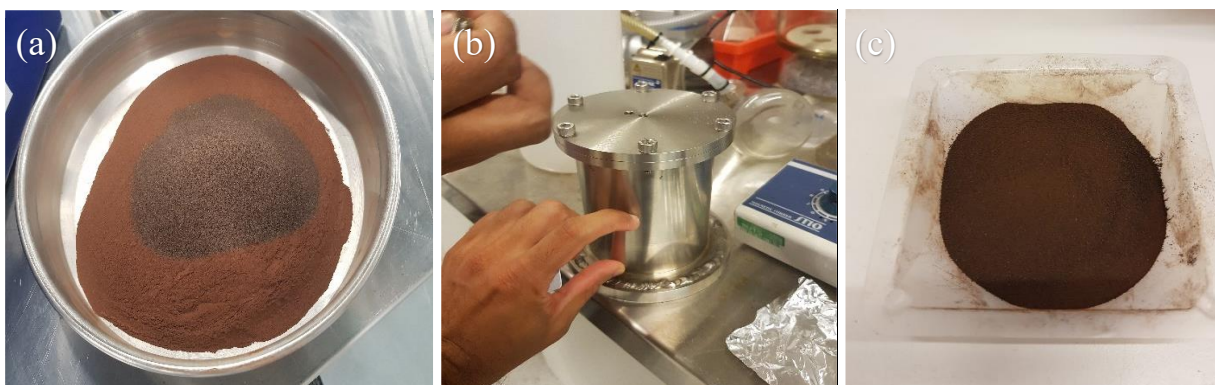
Figure 13. (a) Dried raw sludge powder (b) Pyrolysis reactor (c) WTS-Biochar
