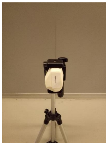
Figure 29 iBeacon set up horizontally
