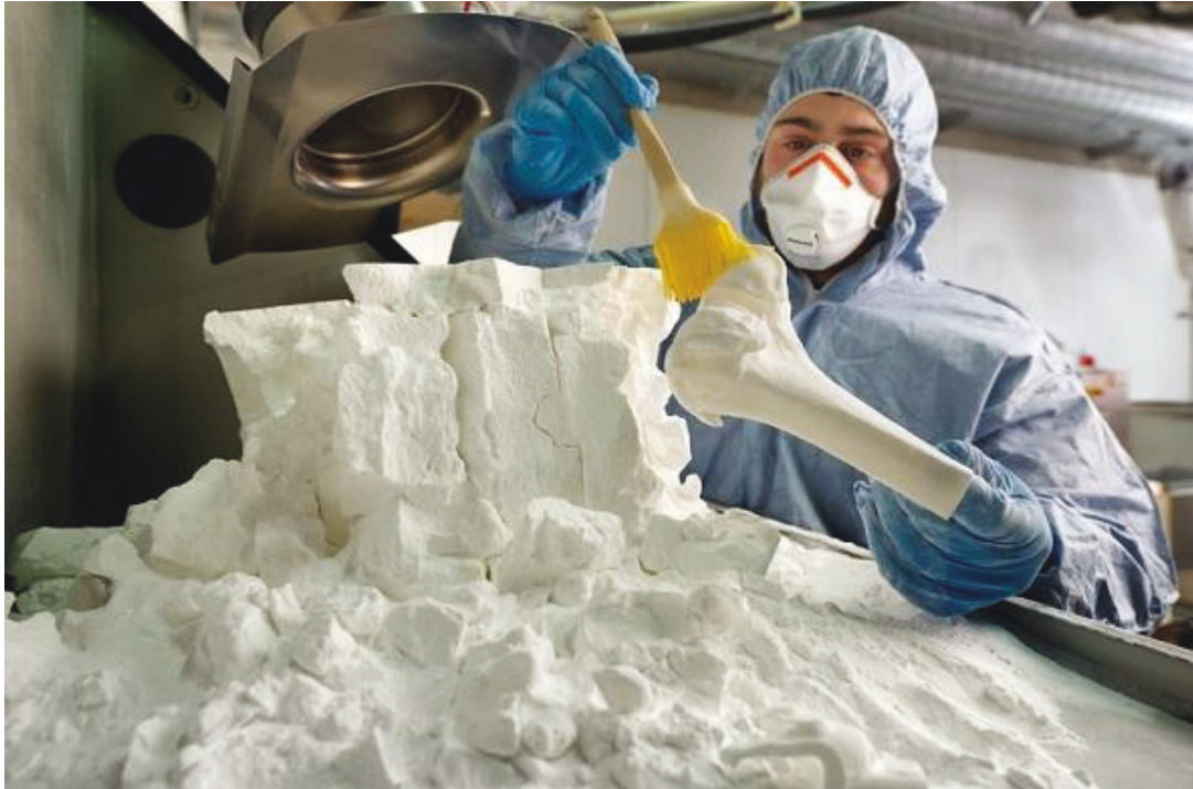
Figure 2.1: General post-processing of an SLS part (courtesy of i.materialise ).
