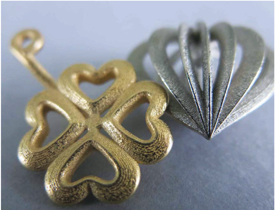
Figure 7.4: Gold and silver broaches showing build steps (courtesy of sculpteo ).
