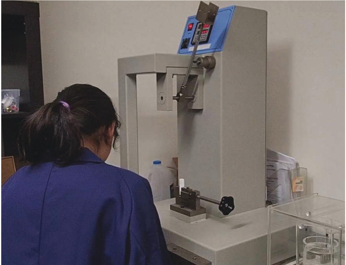
Figure 4.11: Izod test set up at LMATS Pty Ltd.
