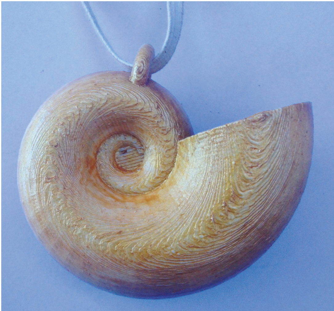
Figure 2.35: 3D printed nautilus shell jewellery piece showing build steps (courtesy of Thingiverse ).
