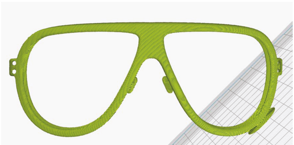
Figure 7.28: Frame with diagonal build steps.
