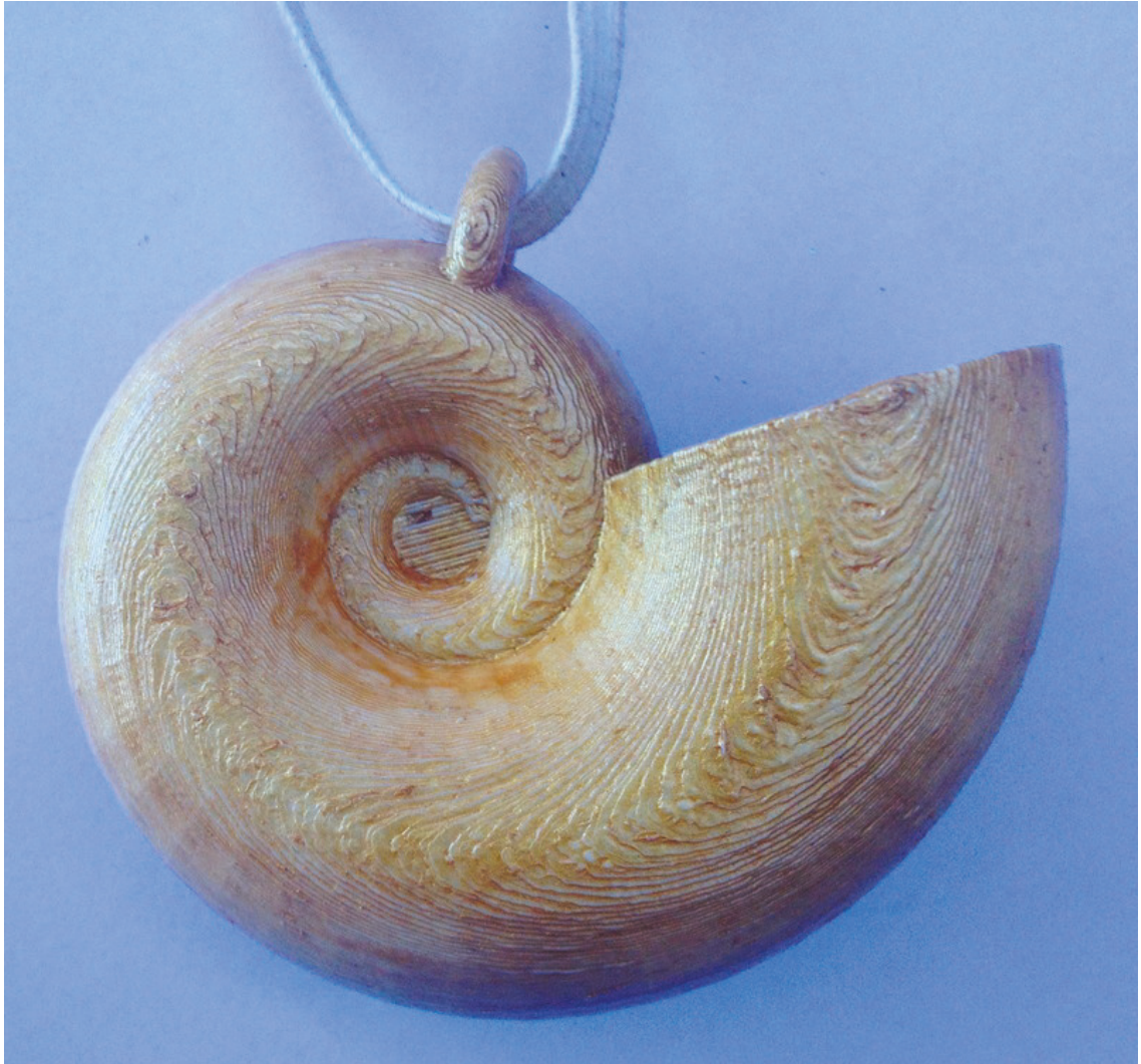
Figure 7.1: 3D printed Nautilus shell pendant showing spiralling build steps (courtesy of Thingiverse ).
