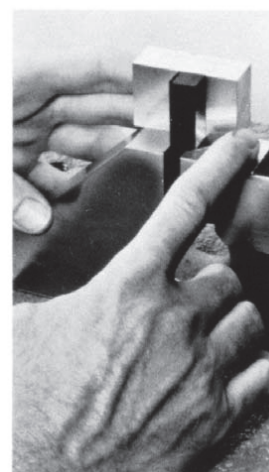
FIG. 4 Jig for Positioning Specimen for Clamping
