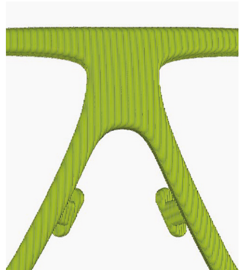
Figure 7.26: Vertical build steps.
