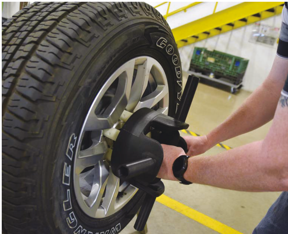
Figure 2.12: 3D printed lug-nut starter tool (courtesy of Eckhart ).
