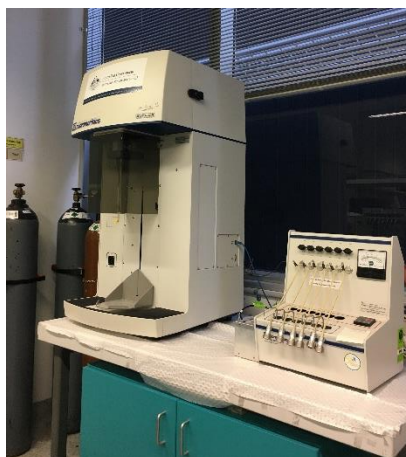
Figure 3.8 The photograph of the Brunauer-Emmett-Teller (BET) used to analyze the samples' surface area during the doctoral study.
