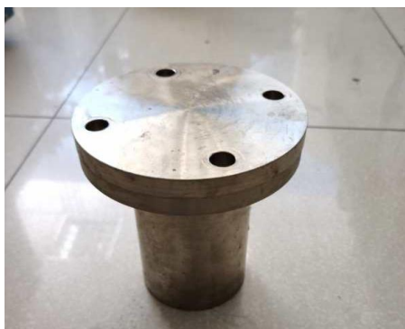
Figure 3.2 The unique designed hydrothermal device, the internal volume is 800 mL.
