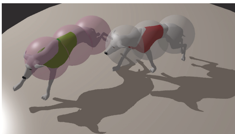
Figure 6.5: Greyhound collision detection using spheres was used in the race simulations.
