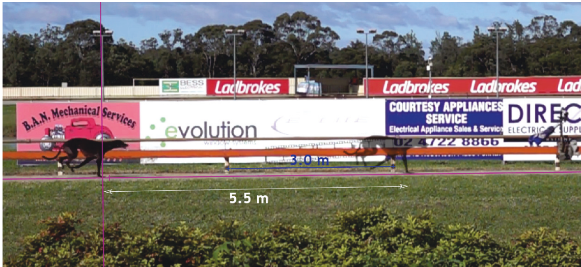
Figure 3.4: HFR video stride analysis using Tracker software for a 500 fps recording.
