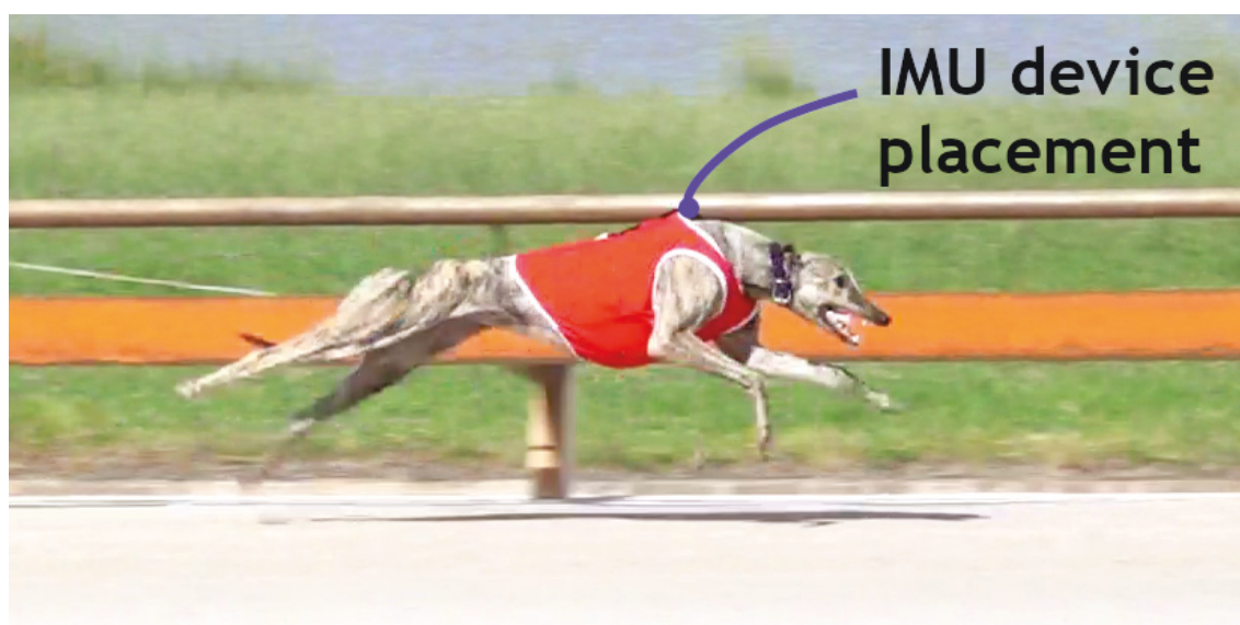
Figure 3.1: Placement of an IMU device inside the jacket of a racing greyhound.
