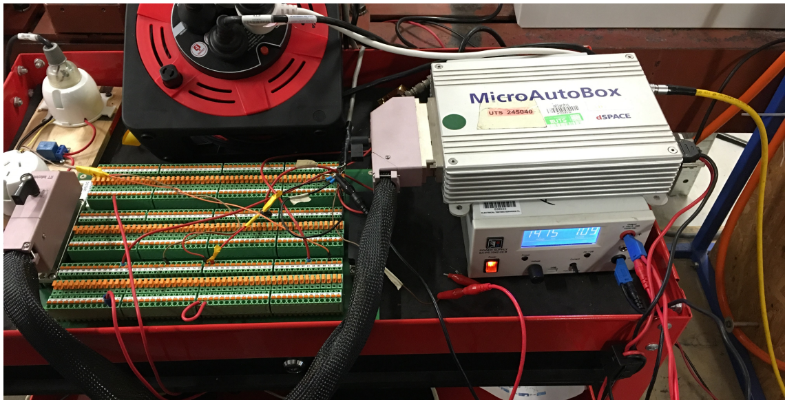
Figure 7.7 : MicroAutoBox and electric control panel
