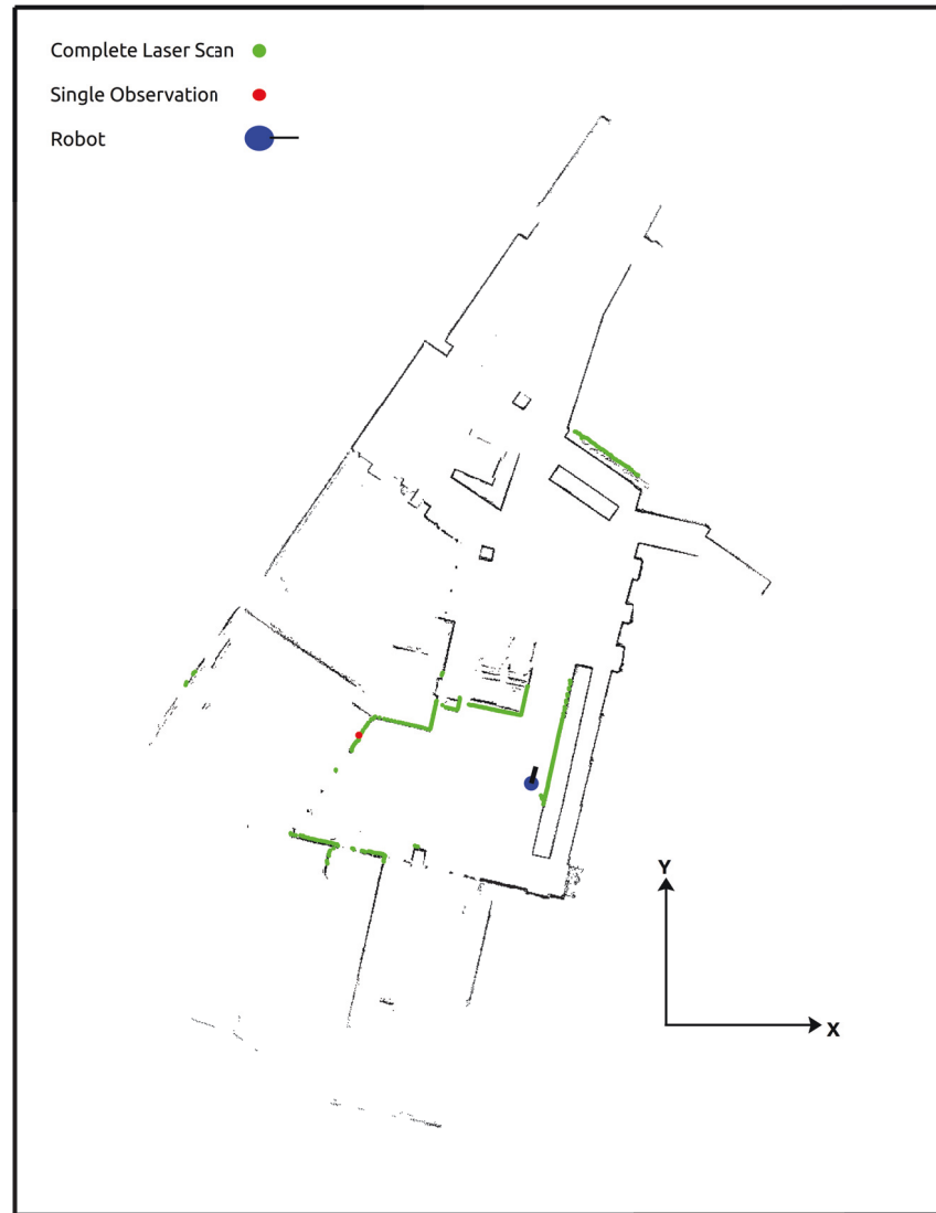
FIGURE 4.8: An example for a laser scan from the Hokuyo 2D LiDAR and the single observation used for active localization
