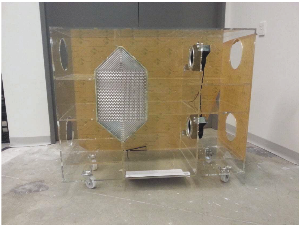
Figure 3.7. Completed Acrylic AHU Casing
