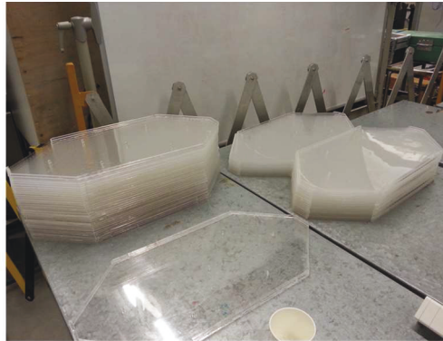
(a) Preparation of the heat exchanger sheets
