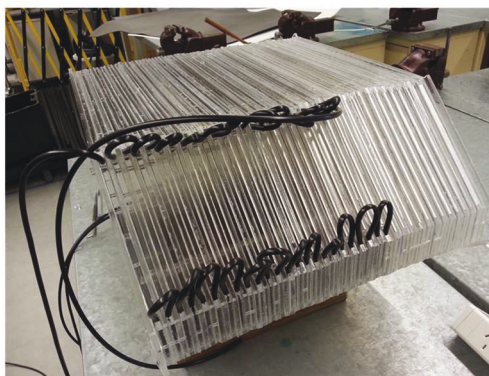
(e) Completed heat exchanger assembly
