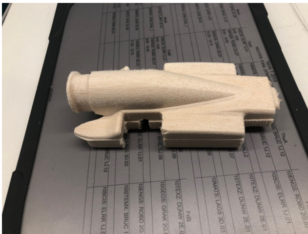
Images 13: car after being milled and ready for competition.
