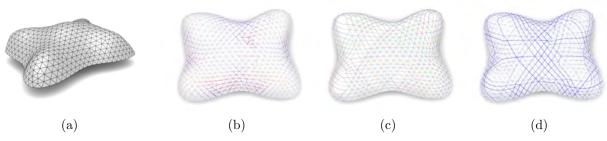
Figure 3: Morphogenesis pipeline: (a) regular remeshing of the input surface; (b) SLS stress on the linear truss model subject to an external load (red compression, blue tension); (c) set of candidate cables; (d) resulting stress on the truss model after the optimization with selected cables and pre-loads.
