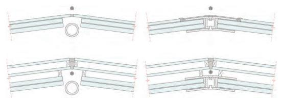
Figure 2: Edge detail with structural laminated glass package, hollow rod as reinforcement (without and with mutual restraint) and spiral cable: (top) with sacrificial glass layer; (bottom) with IGU
