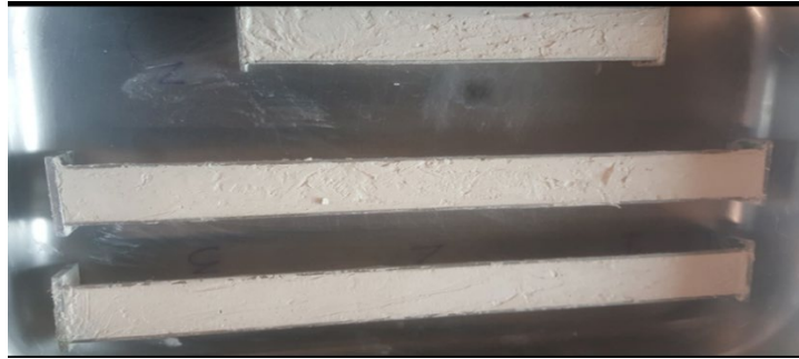
Figure 3.7 and Figure 3.8 illustrate the process of linear shrinkage tests for the treated soil samples with ESP.
