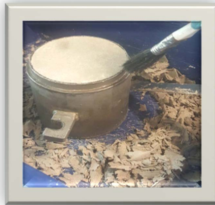
Figure 3.9 Compacted artificial soil sample by adding 5% of eggshell powder
