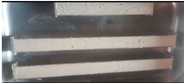
Figure 3.7 Linear shrinkage tests for the treated artificial expansive soil with 5% of the eggshell powder.
