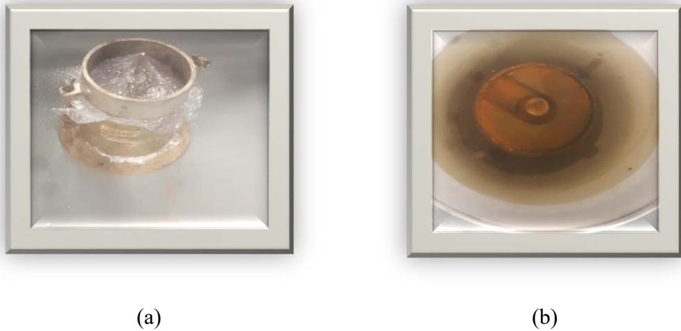
Figure 3.15 CBR sample (a) under the curing condition (b) under the soaking condition
