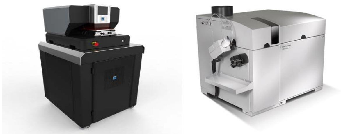
Figure 2.2 NWR-193 Laser Ablation System [123] (left) and Agilent 7700 Series Inductively Coupled Plasma Mass Spectrometer [124] (right).
