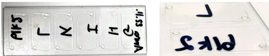
Figure 3.6: Hybriwell™ slide gelatin standards. Plan view and aspect of 2 wells.
