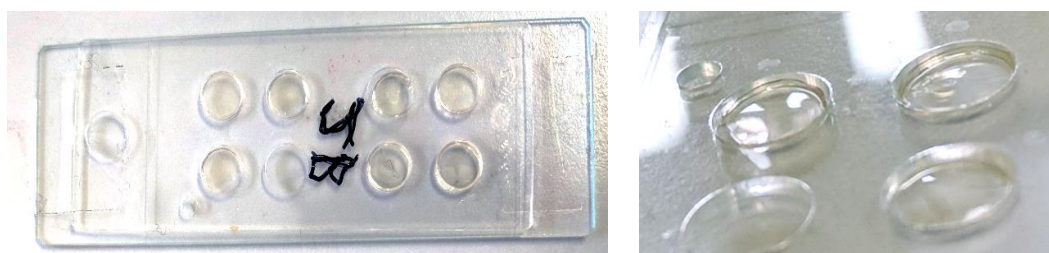
Figure 3.4: Culturewell™ silicon gasket gelatin standards. Plan view and aspect of 4 wells.
