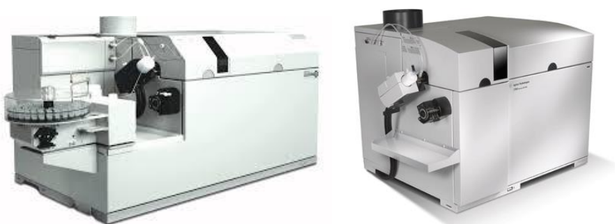
Figure 2.1: Agilent 7500cx (left) and 7700x (right) Series Inductively Coupled Plasma Mass Spectrometer fitted with Agilent Integrated Autosampler [124].
