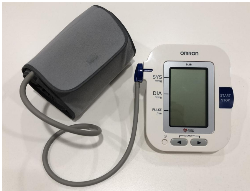
Figure 2.2 shows the Automated blood pressure monitor (Omron IA1B, Japan) used in the present study. The monitor displays systolic and diastolic blood pressure in addition to heart rate data.
