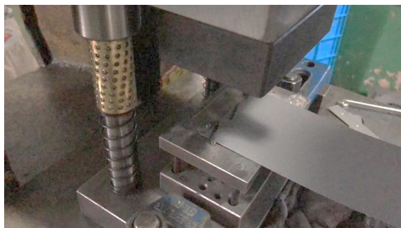
Figure 4-3 Punching process of the silicon steel sheet.
