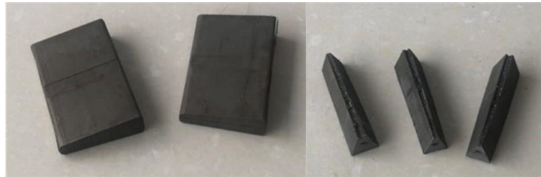
Figure 4-7 Stator and rotor core after wire-electrode cutting.
